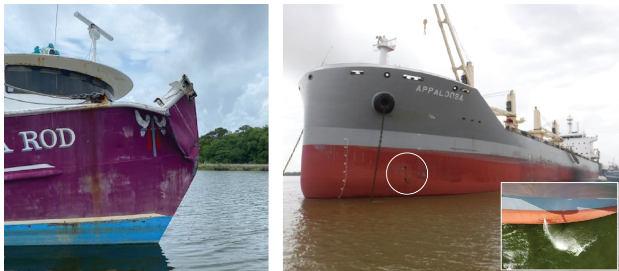
Figure 3. Left to right: Bow damage to the Papa Rod , and Appaloosa hull breach (circled). Right inset shows ballast water leaking from the breached hull. (Source: US Coast Guard)
