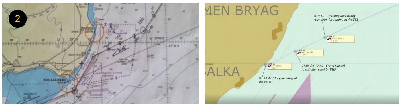
FIGURE 2 PART OF THE PASSAGE PLAN AROUND THE STRANDING DRAWN BY 2ND OFFICER ON A NAVIGATIONAL CHART AND AIS PLOTS SHOWING FINAL STAGES OF THE SHIP'S PASSAGE
