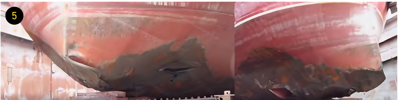
FIGURE 5 DAMAGES OF THE SHIP IN THE BOW (PORT AND STARBOARD) SOURCE REPUBLIC OF BULGARIA NAMRAIB
