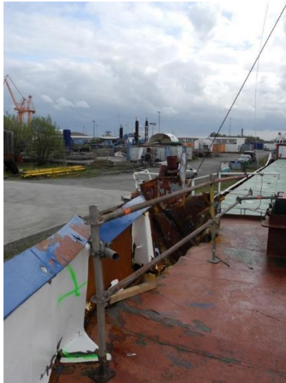
Figure 5: Forecastle with view of the damage 6
