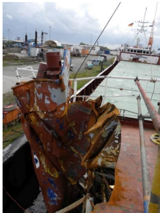
Figure 6: Rippled hull plating at the breach 7
