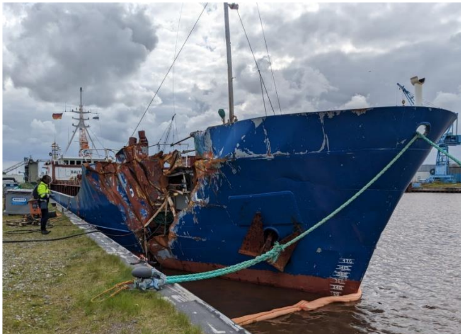
Figure 3: Damage to the bow 4
