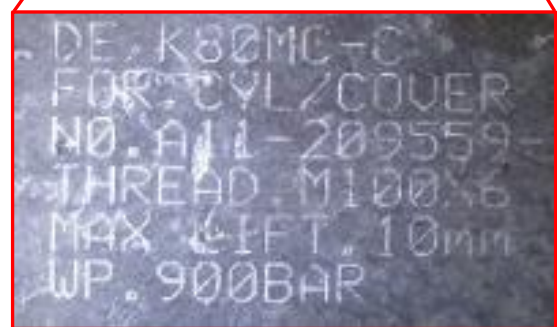
Figure 5: Maximum working pressure and lift, stamped on the hydraulic jack assembly
