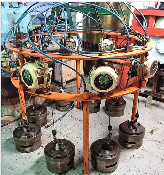
Figure 2: Hydraulic jack assembly used to untighten the cylinder head
