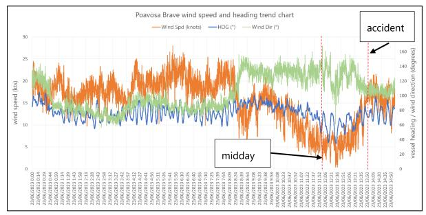
Figure 7: Wind speed, direction and vessel heading data from the vessel's ECDIS
