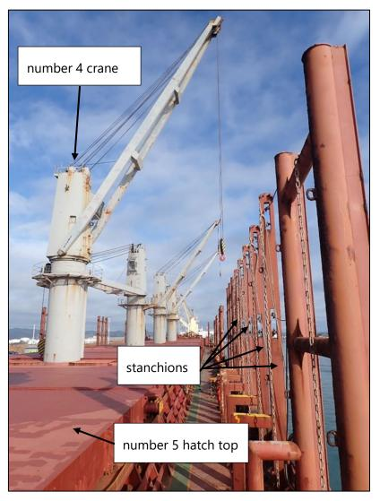
Figure 4: Starboard stanchions, raised position
