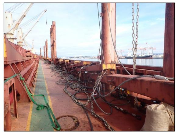
Figure 3: Starboard stanchions, lowered position
