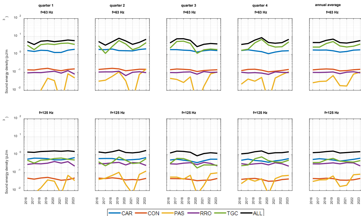
Figure 46 Sound energy density (in \text{pJ/m}^3 ) of different vessel categories for each quarter and year in the Northeast Atlantic Ocean. The top panel is for 63 Hz. The bottom panel is for 125 Hz.
