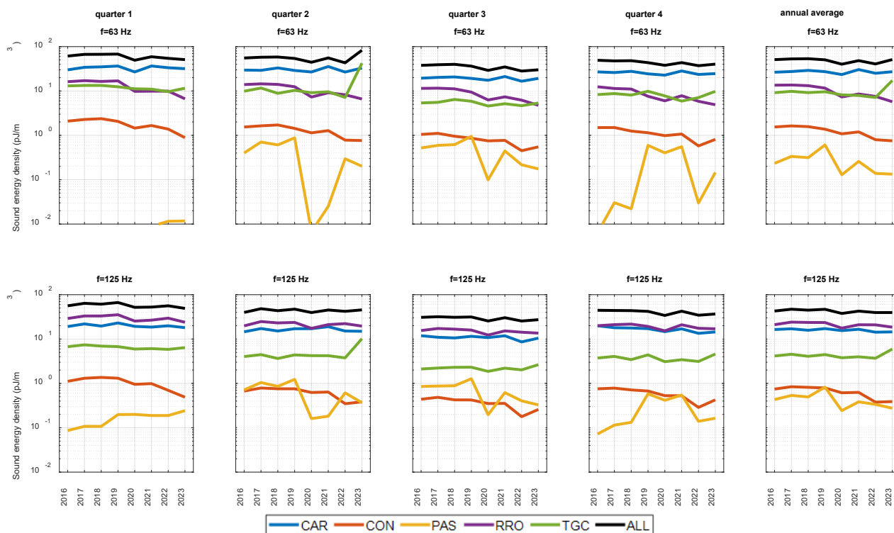
Figure 24 Sound energy density (in pJ/m 3 ) of different vessel categories for each quarter and year in the Baltic Sea. The top panel is for 63 Hz. The bottom panel is for 125 Hz.
