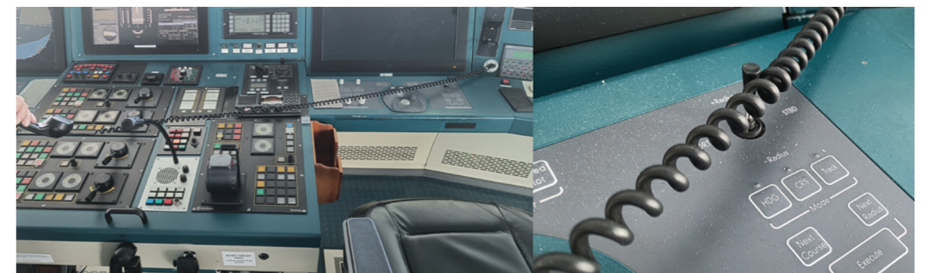
FIGURE 48. Bridge centre console telephone cable mingling with the track pilot joystick
