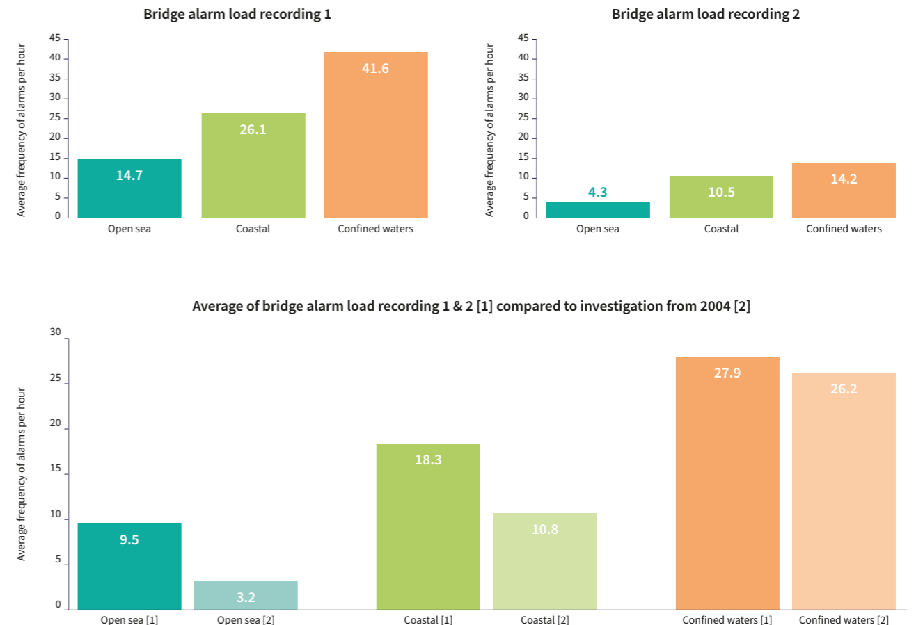
FIGURE 28. Three column charts illustrate the average alarm load on the bridge per hour, at open sea, in coastal areas, and in confined waters, as well as a comparison of the alarm load observed by the authors and the alarm load observed in 2004 by F. Motz and M. Baldauf [69]
