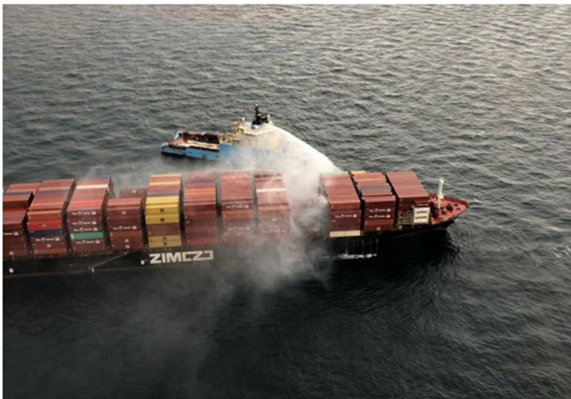
Figure 3. Maersk Trader performing boundary cooling (Source: Resolve Marine)
