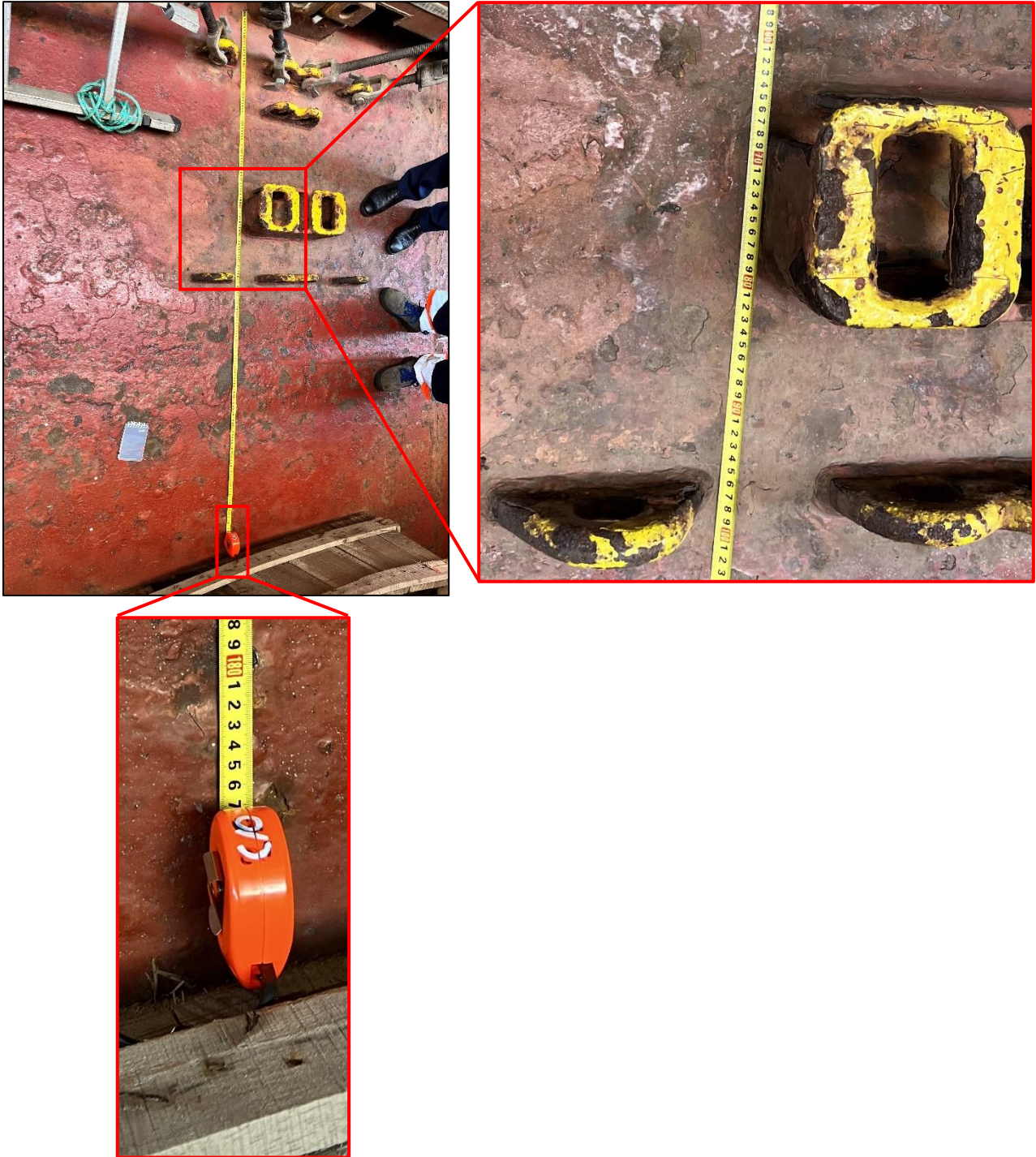
Figure 5: The measured width of the cross deck between the accommodation superstructure and bay 46
