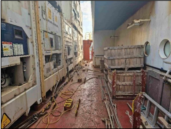
Figure 5: The cross deck (as seen from the port side), during cargo operations in the bay and when the reefer containers are lashed in
