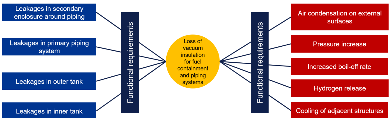
Figure 8-4 Loss of vacuum insulation for liquefied fuel containment and piping systems (High-level bow tie illustration).
