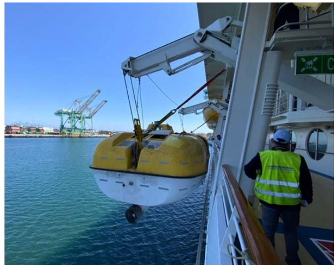
A drill with a davit-launched lifeboat
