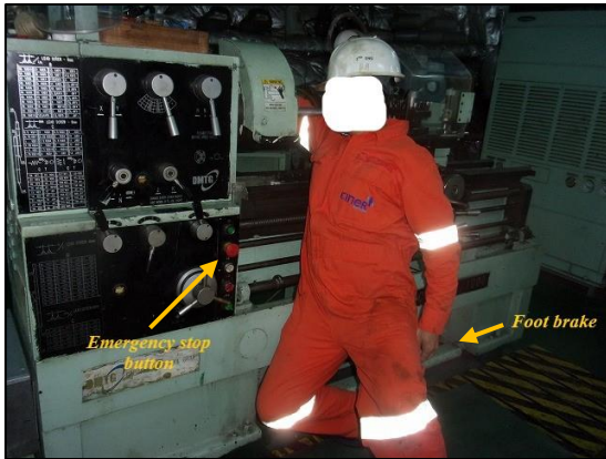
Figure 7: Simulation of the accident, showing how the fitter's body was pulled into the lathe
