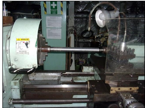
Figure 4: The securing pin placed in the lathe
