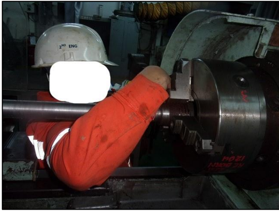
Figure 6: Simulation of the accident, showing how the fitter's hand was pulled towards the chuck
