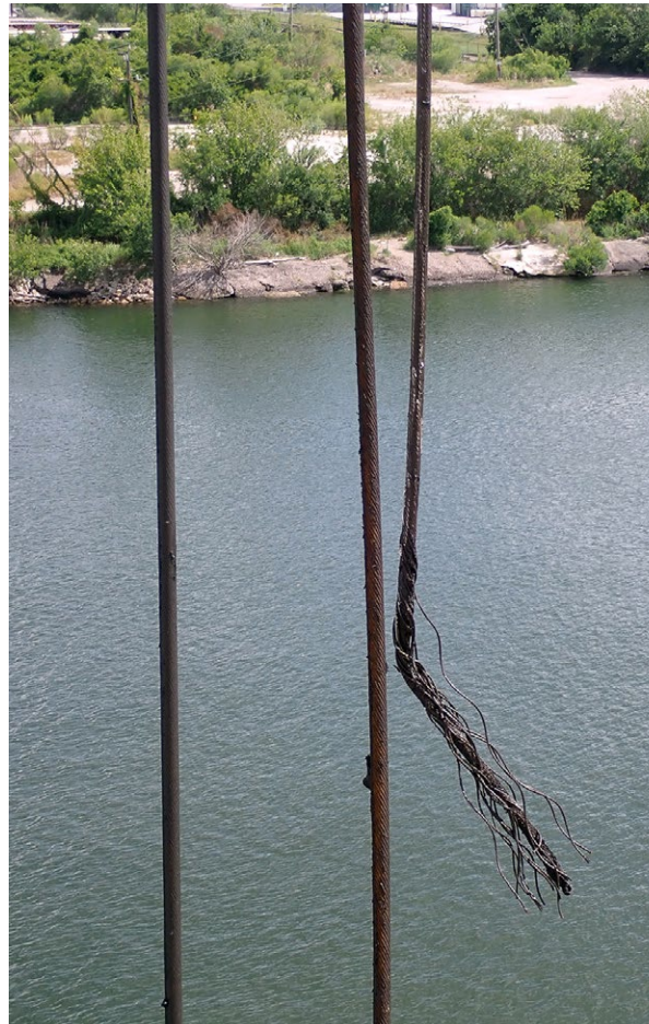
Left to right: Crane no. 1's parted wire rope on the crane side and its block smashed into the top of the damaged nacelle. SOURCE: COAST GUARD
