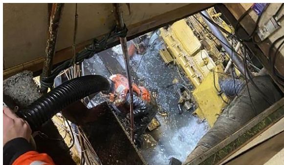
Looking down into the engine room of the Captain Alex at 0326, with the water midway up the starboard main engine and the captain of the vessel on the stairs. The suction hose to the portable dewatering pump (on deck) is on the left. SOURCE: COAST GUARD
