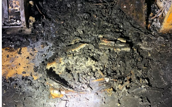
Remains of the lithium-ion and nickel-metal hydride battery chargers on the communications table.
