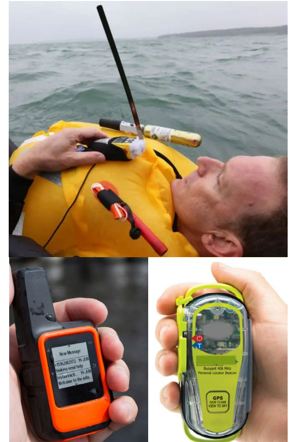
Clockwise from top: PLB attached to lifejacket, exemplar PLB, and SEND. SOURCES: VAREN, POWERANDMOTORYACHT.COM, AND BLUEWATERSAILING.COM
