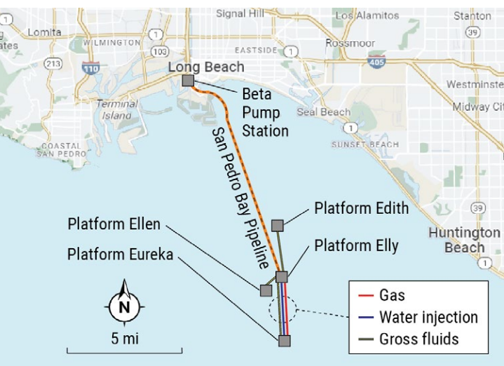
Simplified illustration of the San Pedro Bay Pipeline and supporting structures. BACKGROUND SOURCE: GOOGLE MAPS
