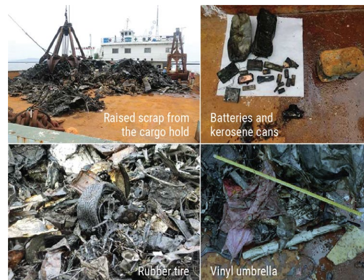
Photos from a Japan Transportation Safety Board report on a scrap metal fire in a moored vessel's cargo hold, showing the scrap metal raised from the cargo hold and the nonmetal material mixed in with the scrap metal.
