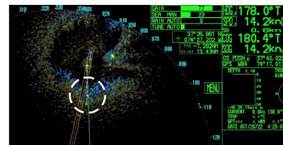
Tremont (circled) crossing ahead of MSC Rita at 0029:17 as seen on the containership's X-band radar.
