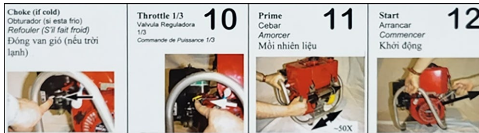
A P6 pump like the one sent to the Captain Alex showing the priming handle and cap. SOURCE: COAST GUARD
