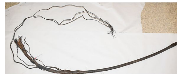
Thorco Basilisk parted hoisting wire rope (crane side of fracture). SOURCE: ENGINEERING SYSTEMS INC
