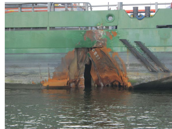
Damage to the aft port side of the Thunder . SOURCE: COAST GUARD
