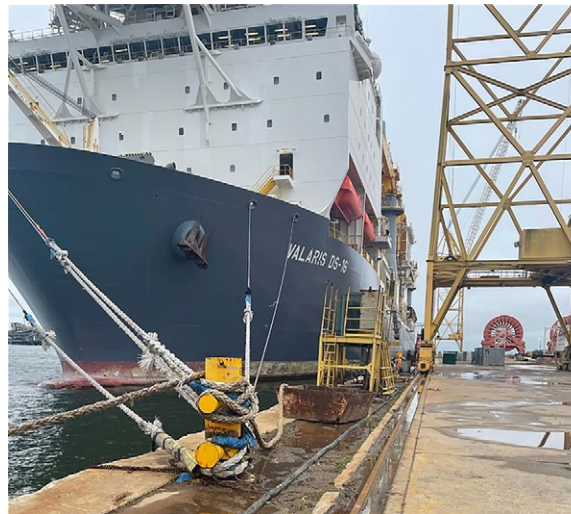
VALARIS DS-16 moored at STEHMO Shipyard at unknown date before the casualty with lines secured to bollard 6 (before lines were adjusted for the March 12 strong winds). SOURCE: VALARIS DS-16 CAPTAIN
