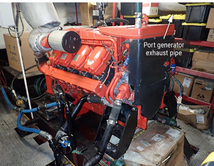
Photo from survey on June 2, 2022, showing port main engine (foreground) and storage shelf. The white port generator exhaust pipe is visible behind some of the boxes on the shelves.
