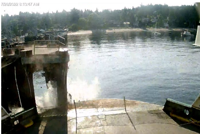
Still image from forward-looking camera footage on board the Cathlamet at the time the ferry's port bow struck the dolphin.
