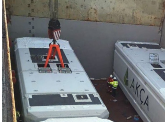
Exemplar Nordex Delta 4000 wind turbine nacelle in another vessel's cargo hold rigged in accordance with manufacturer-recommended guidance. SOURCE: NORDEX
