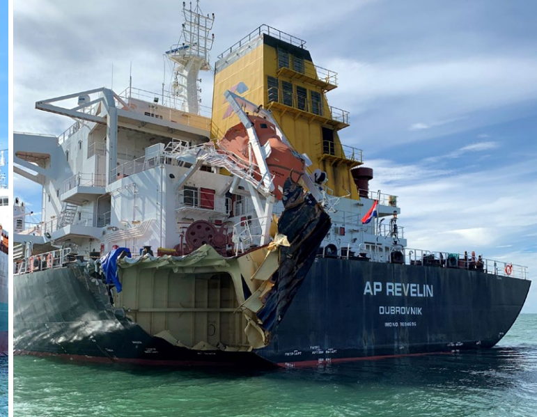
Left to right: Port bow of the Damgracht and damaged stern area of the AP Revelin after the collision. SOURCE: NTSB
