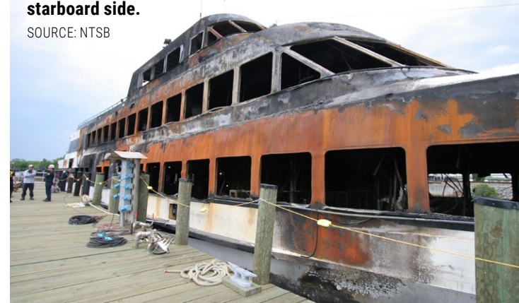
Exterior damage to the Spirit of Norfolk , starboard side.
