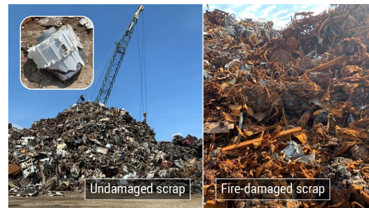
Cargo removed from CMT Y Not 6 postfire. Left: Scrap metal unaffected by the fire; rubber tires and other nonmetallic materials are visible. Inset: A washing machine drum shrouded in plastic. Right: Scrap metal exposed to the fire, with large metal pieces of solidified molten metal. SOURCE: NTSB
