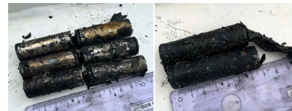
Left to right: Remains of the nickel-metal hydride and the lithium-ion battery cells and components found on the communications table. SOURCE: ATF
