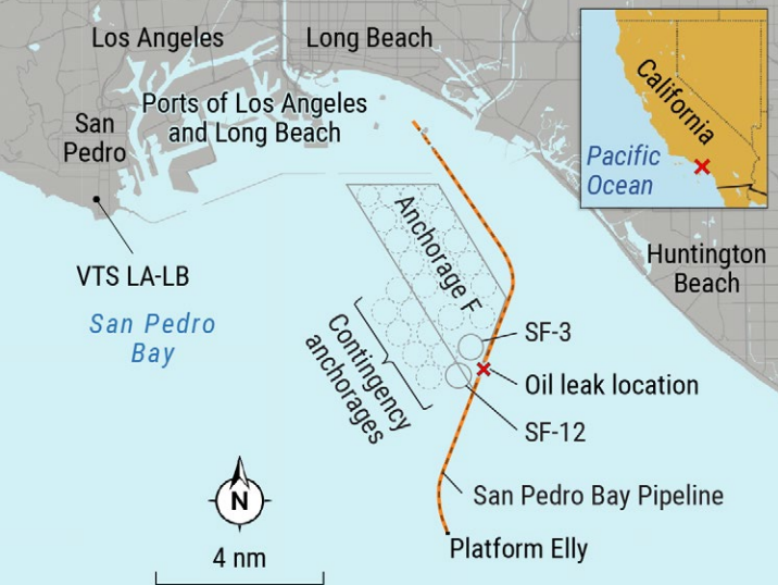
San Pedro Bay Pipeline, with locations of oil release, federal Anchorage F, and contingency anchorage positions near Anchorage F.
