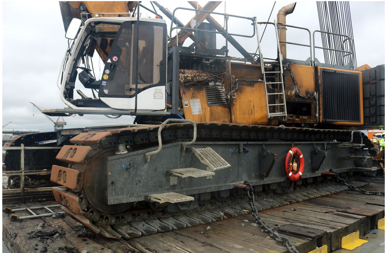
The damaged crane postfire. SOURCE: COAST GUARD
