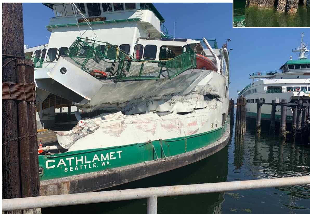
Below: The damaged Cathlamet after the contact with the dolphin. Right: The damaged dolphin. SOURCE: WSF
