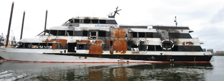
Exterior damage to the Spirit of Norfolk port side after the fire. The engine room ventilation openings are circled. SOURCE: NTSB
