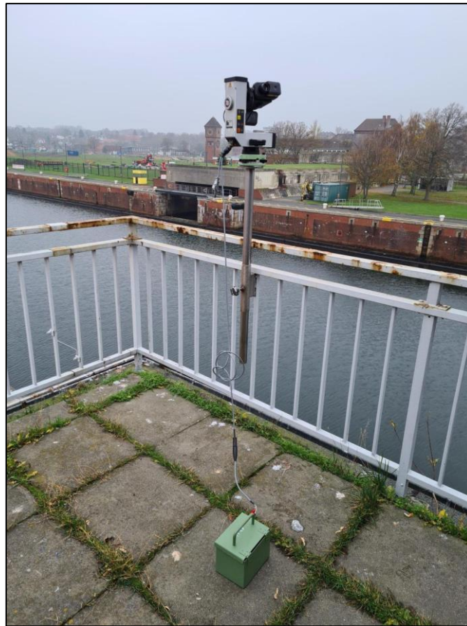
Figure 41: Altimeter in pre-installed holder 55
