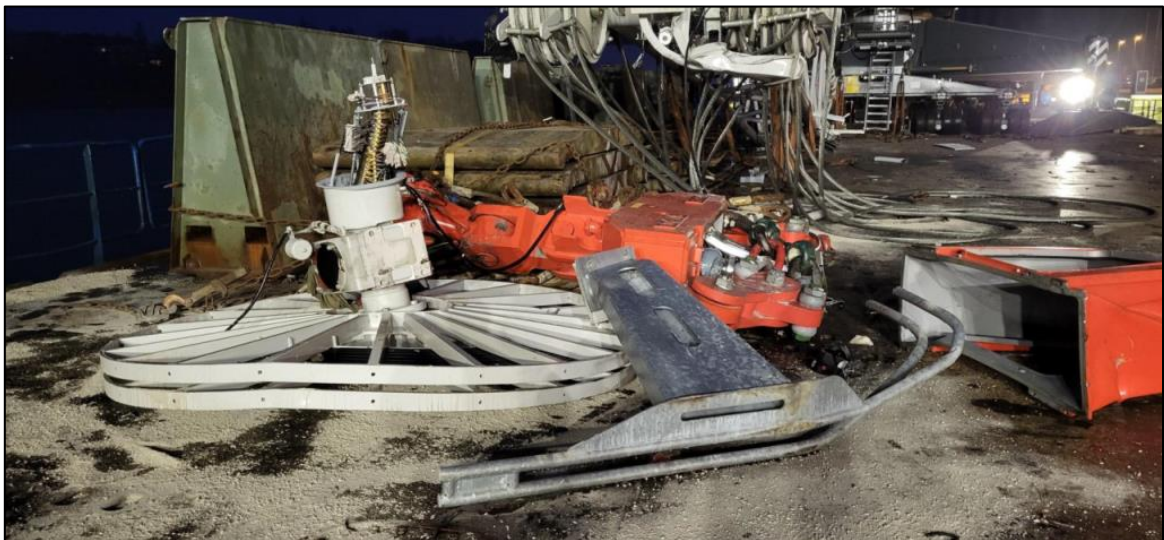
Figure 10: Remnants of some attachments from the jib 18
