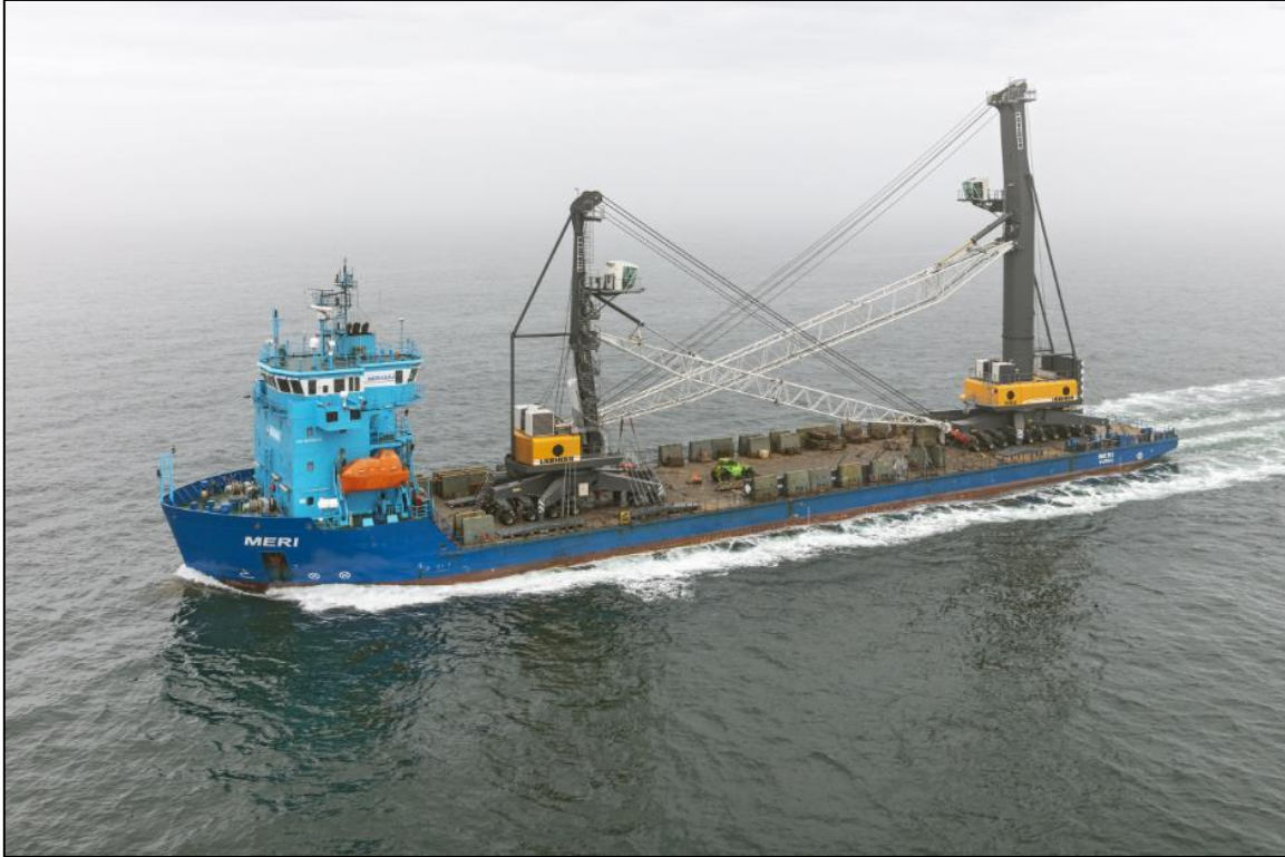
Figure 1: The MERI laden with two mobile harbour cranes. 4
