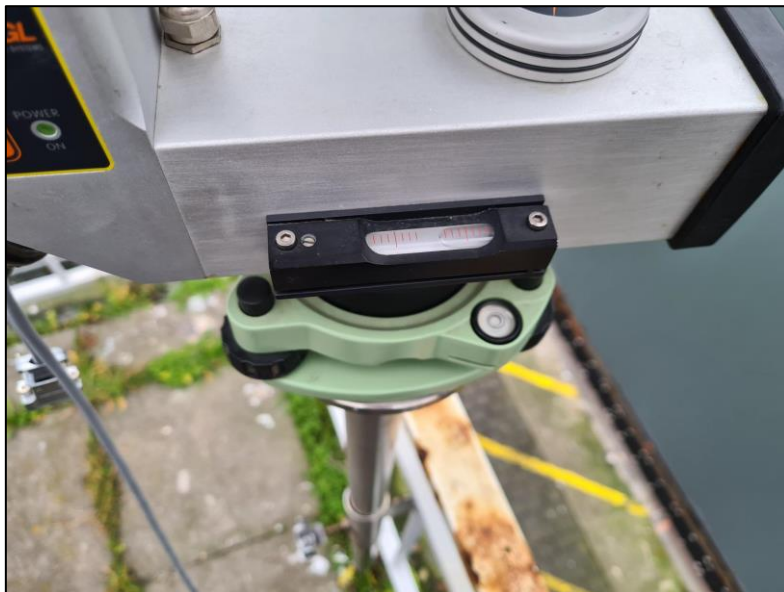
Figure 43: Altimeter levelled using a spirit level 57
