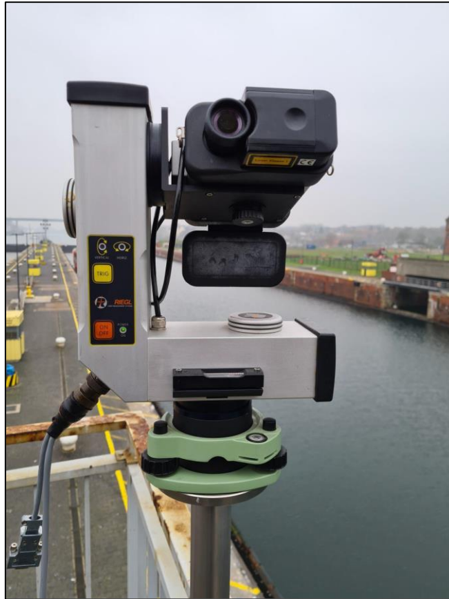
Figure 42: Altimeter mounted and ready for operation 56
