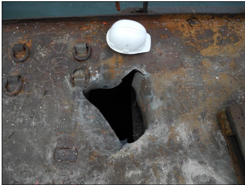
Figure 11: Penetrated deck 19 The helmet is used for size comparison.
