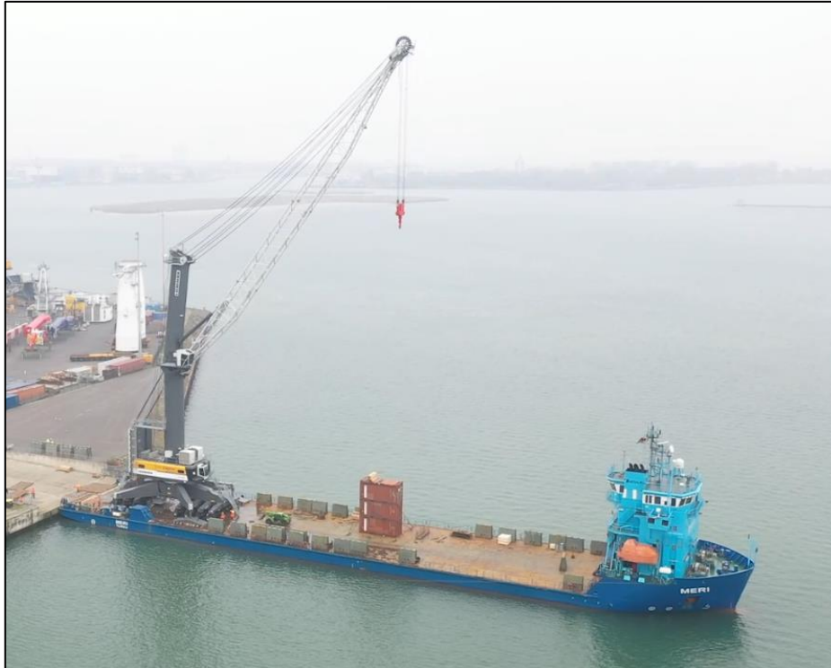
Figure 36: Loading the LHM 600 Evo6 onto the MERI 40
