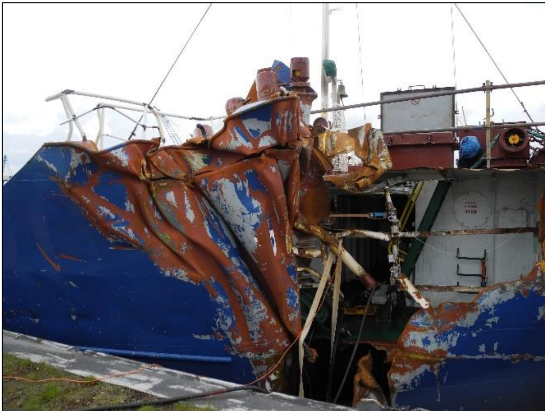
Figure 6: Torn open side of the PETRA L 12
