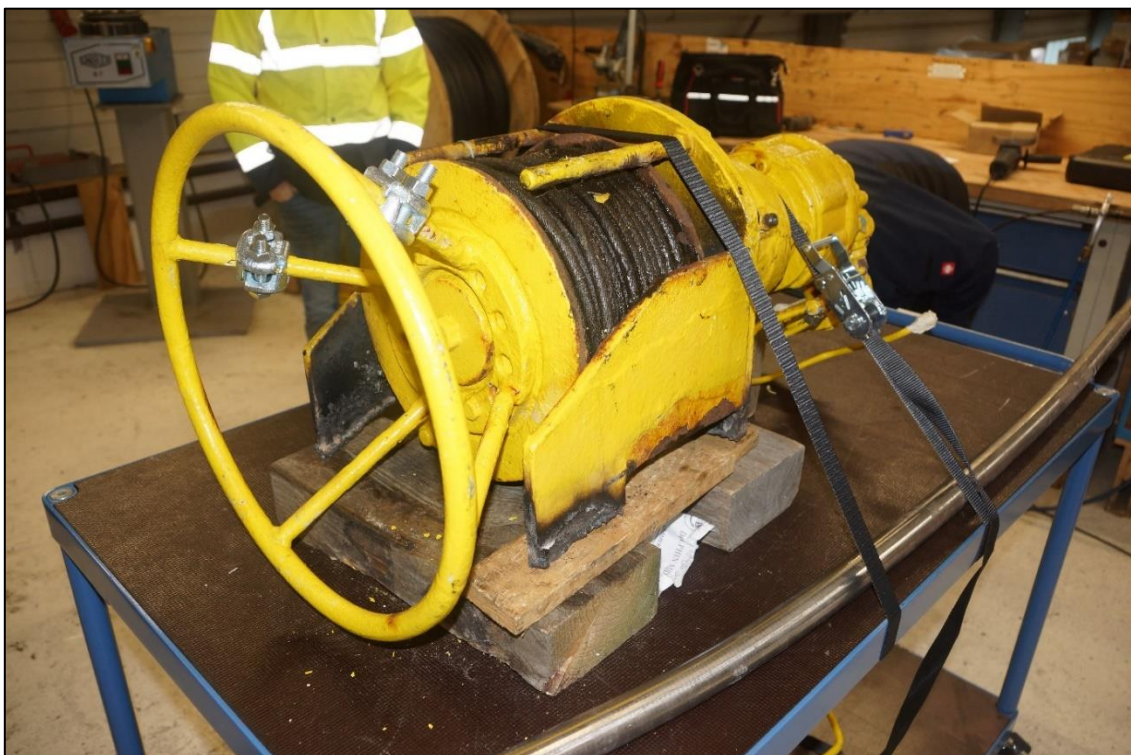
Figure 12: The dismantled cable winch before it was disassembled 18
