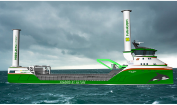
Rendering of cargo ship With Orca to be powered solely by green hydrogen, wind, and on-board batteries for use in the North Sea.
