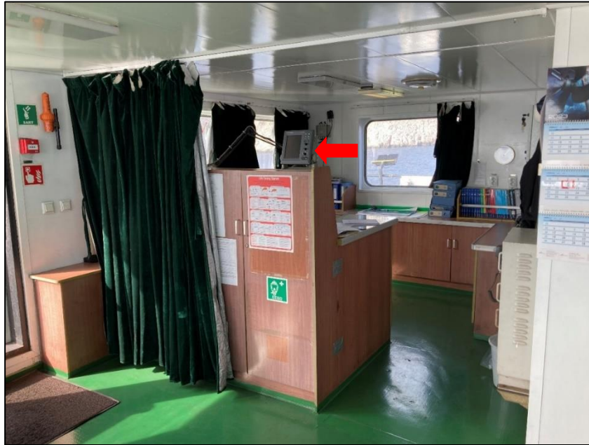
Figure 4: The chart room, as seen from forward (red arrow: echo sounder display)
