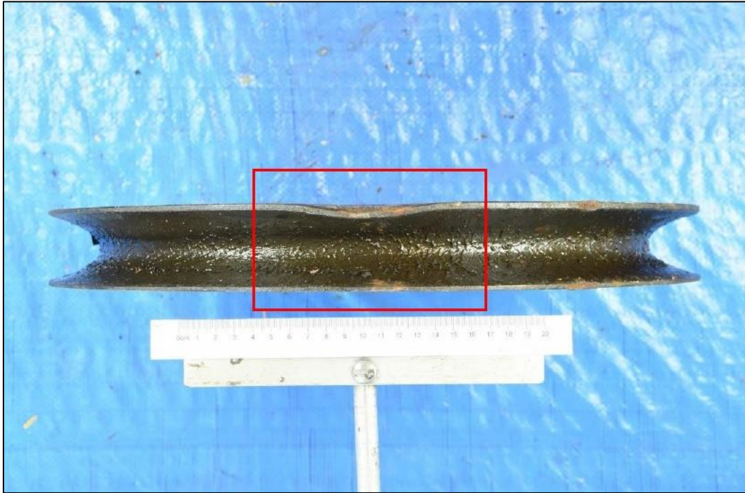
Figure 21: The deformation on the crane's sheave Source: Failure Analysis Report
