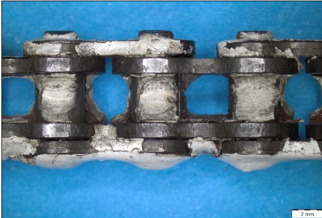
Figure 18: Microscopic view of the drive chain, with the adherent white paint visible Source: Failure Analysis Report
