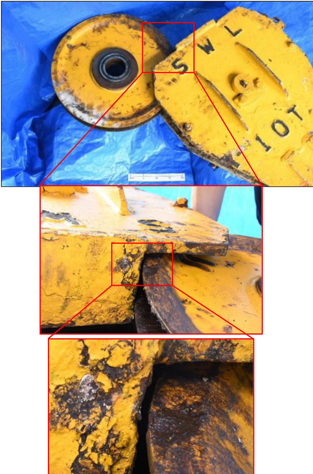
Figure 23: The point of contact between the block and the crane's sheave Source: Failure Analysis Report
