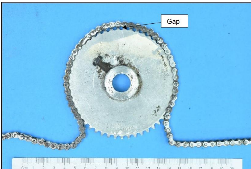
Figure 19: Gap between the drive chain and the small sprocket Source: Failure Analysis Report
