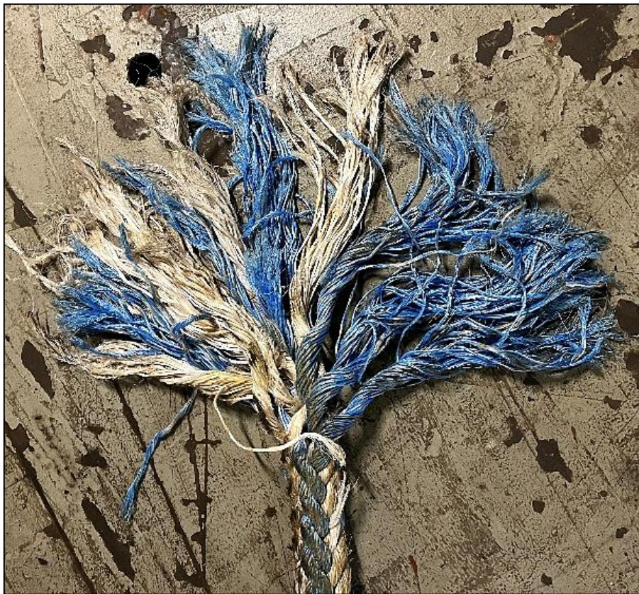
Figure 9: The point of failure
