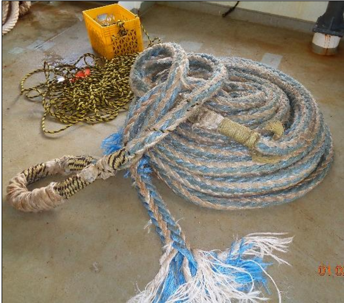
Figure 6: The forward spring line that parted
