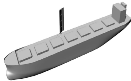
Single FastRig installed on the vessel
