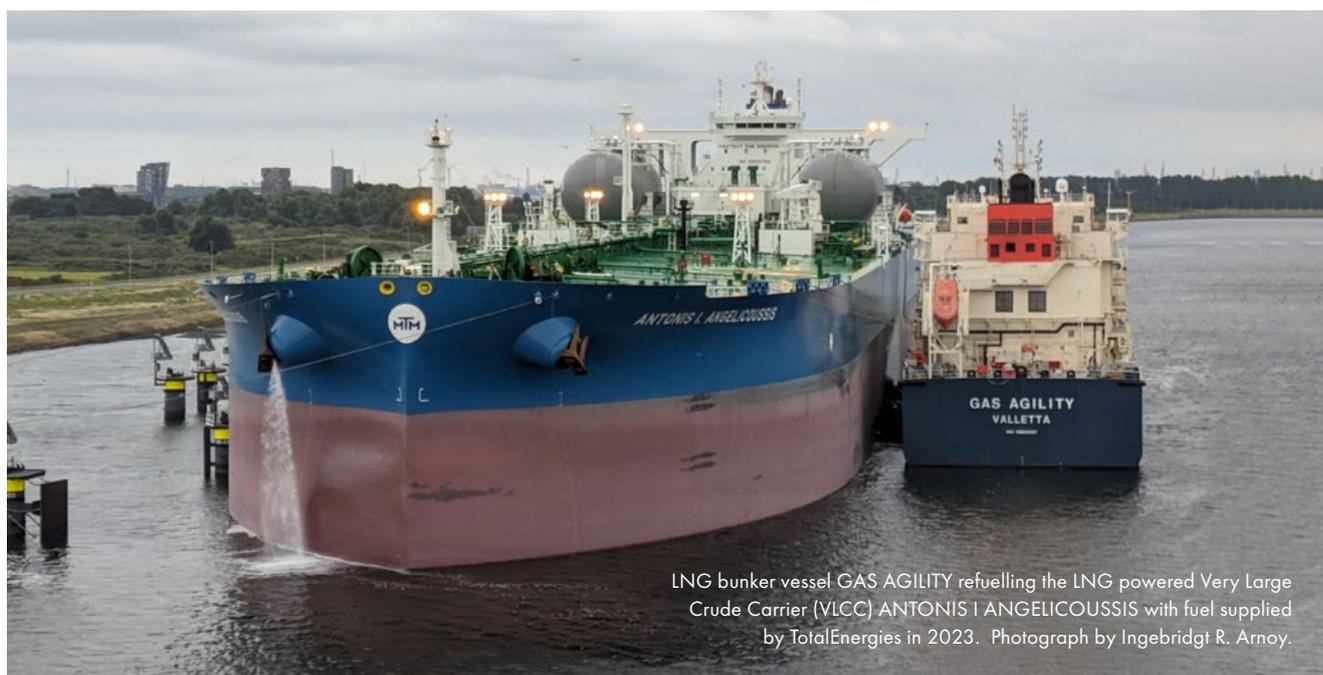
LNG bunker vessel GAS AGILITY refuelling the LNG powered Very Large Crude Carrier (VLCC) ANTONIS I ANGELICOUSSIS with fuel supplied by TotalEnergies in 2023. Photograph by Ingebridgt R. Arnoy.
