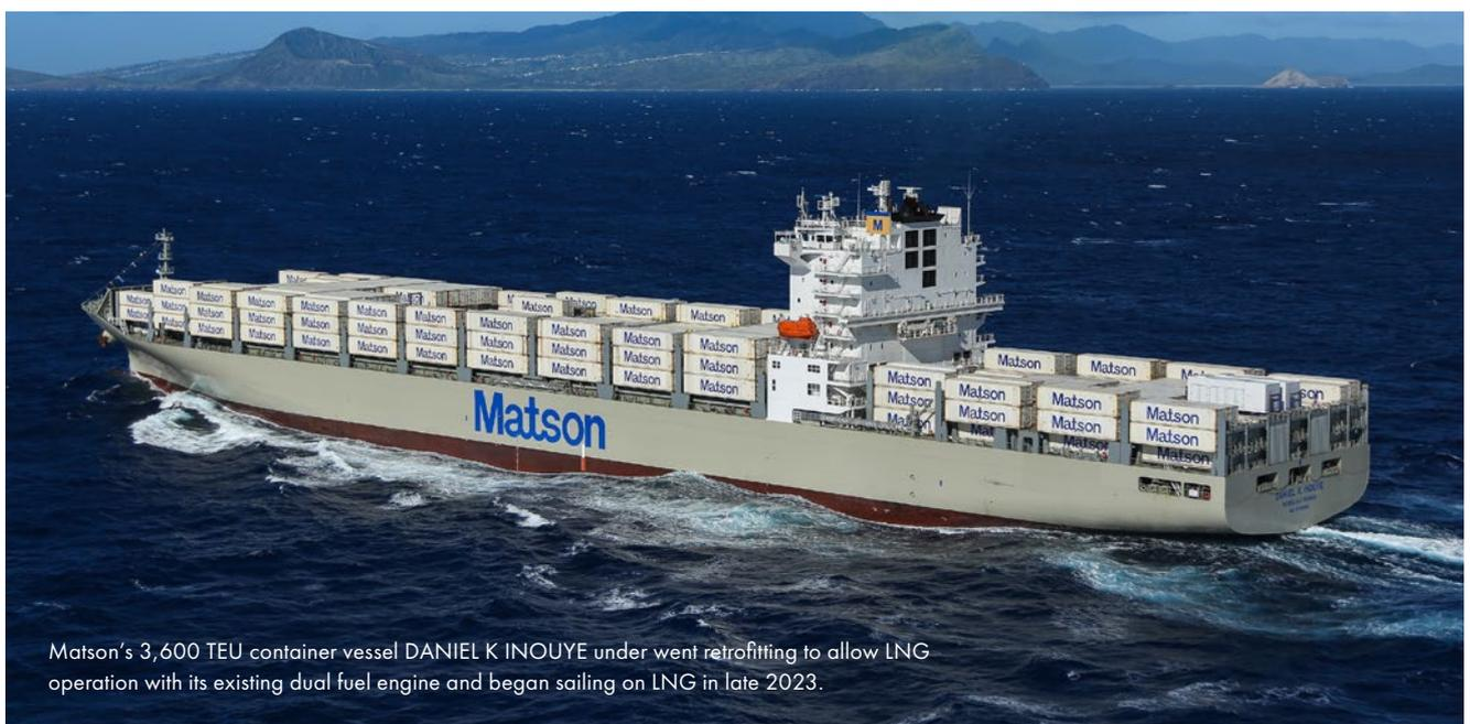
Matson’s 3,600 TEU container vessel DANIEL K INOUYE underwent retrofitting to allow LNG operation with its existing dual fuel engine and began sailing on LNG in late 2023.
