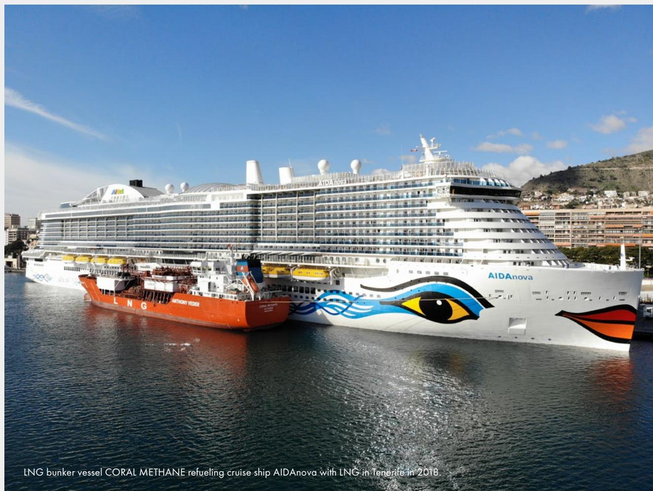
LNG bunker vessel CORAL METHANE refueling cruise ship AIDAnova with LNG in Tenerife in 2018.
