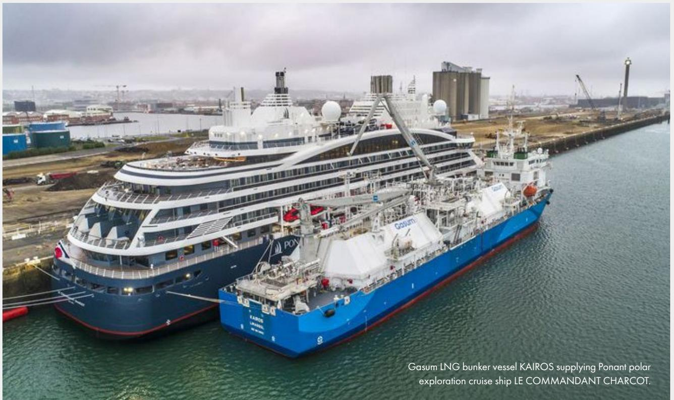
Gasum LNG bunker vessel KAIROS supplying Ponant polar exploration cruise ship LE COMMANDANT CHARCOT.
