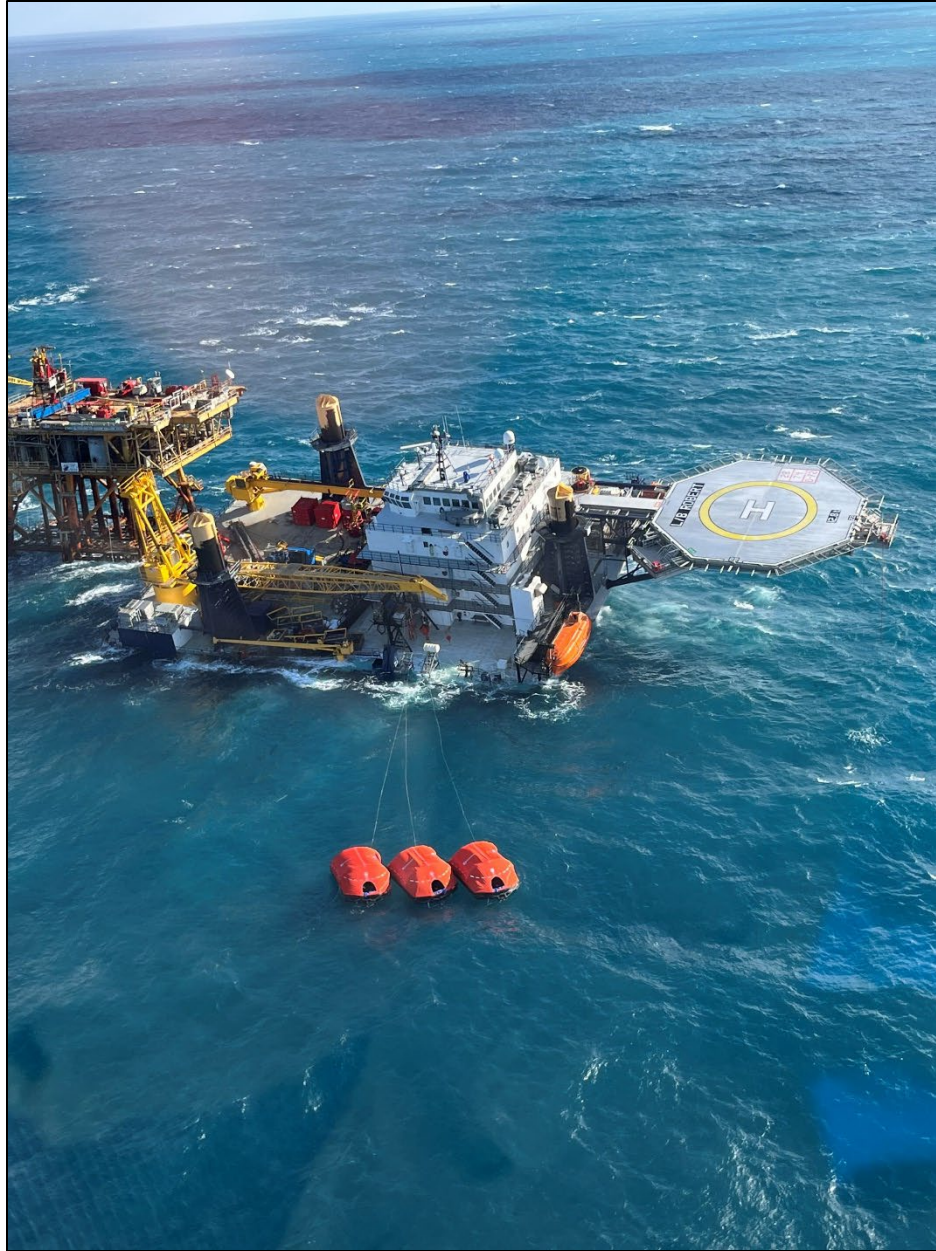
Figure 5. L/B Robert tilting to port as seen on November 21, 2022, at 0914. (Source: Coast Guard)
