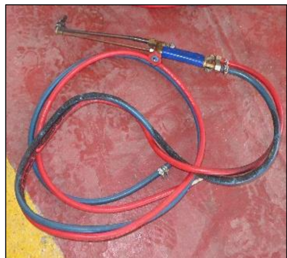
Figure 4: Heat damages on the section of the oxy-acetylene hoses closest to the torch
