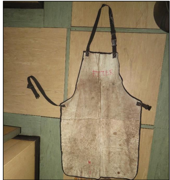
Figure 7: The hot work apron worn by the fitter
