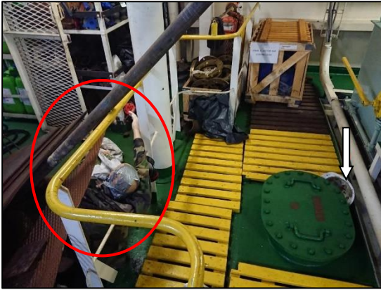
Figure 4: Simulation of how the second engineer was found (red circle); the second engineer's safety helmet can be seen near the manhole, to the left (white arrow)
