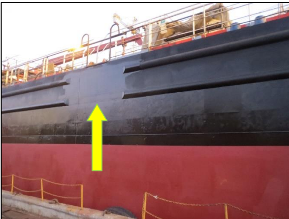
Figure 8: alterations to the vessel's shipsides, showing the removal of the rubbing strakes in way of the starboard side pilot station
