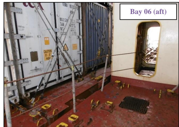
Figure 3: Stanchions and rope fitted on the aft side of bay 06 and passing through crane no. 1's platform
