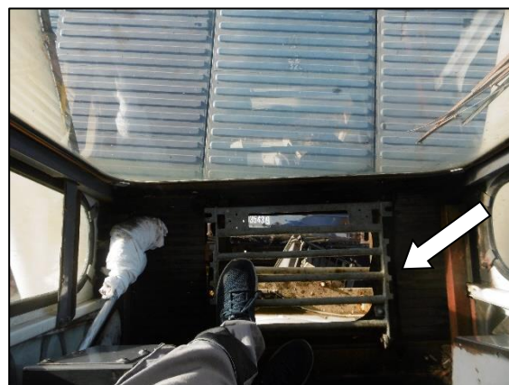
Figure 8: Maintenance access hatch inside the deck crane's cabin
