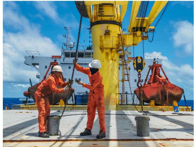
Crew changing wire
