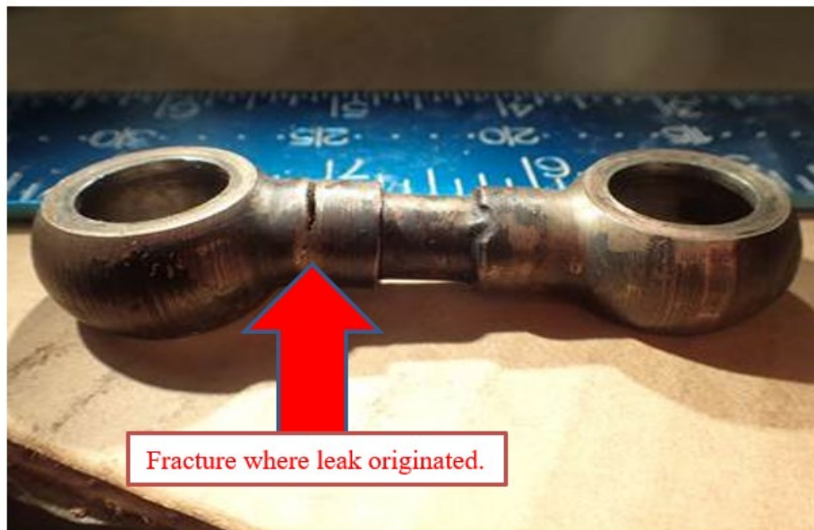
Figure 8. The fractured banjo tube. (Source: QC Metallurgical, Inc.)
