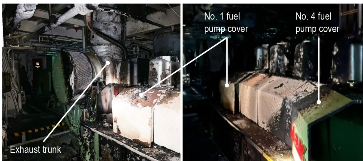
Figure 3. (Left) Location of the turbo charger relative to the no. 1 fuel pump cover. (Right) Location of fire on the starboard engine with fuel pump covers nos. 1 and 4 left partly opened. (Source: US Coast Guard)
