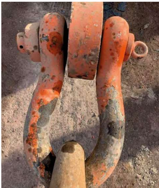
Deformed shackle pin in pulling arrangement
