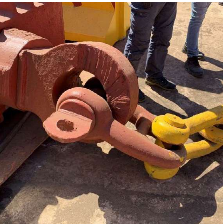
Crudely modified components in pulling system
