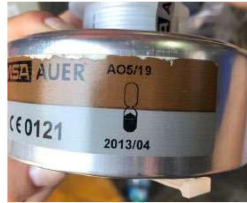
All filters stored in the emergency room had expired Site Inspection Report of Blade (13.1.2023)
