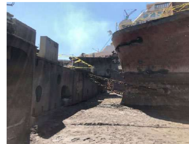
Aft part of the ship cut off on the beach
