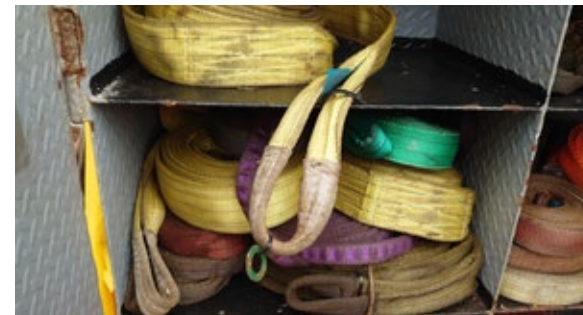
! Webbing slings with green tags – colour indicating the last annual inspection performed.
