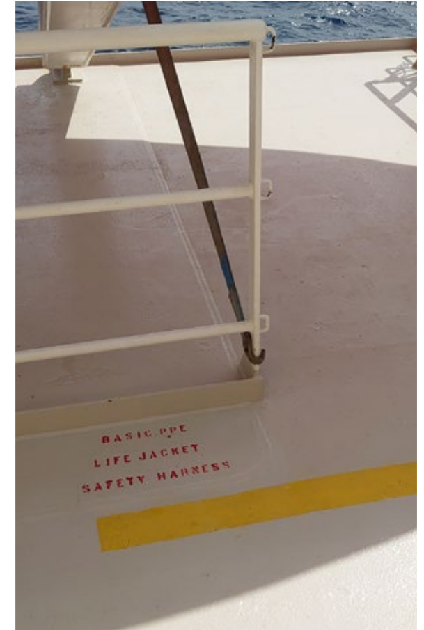
! This operator uses colour-coded lines to indicate PPE requirements. In this case, basic PPE + lifejacket + fall protection equipment are required when moving beyond the yellow line.
