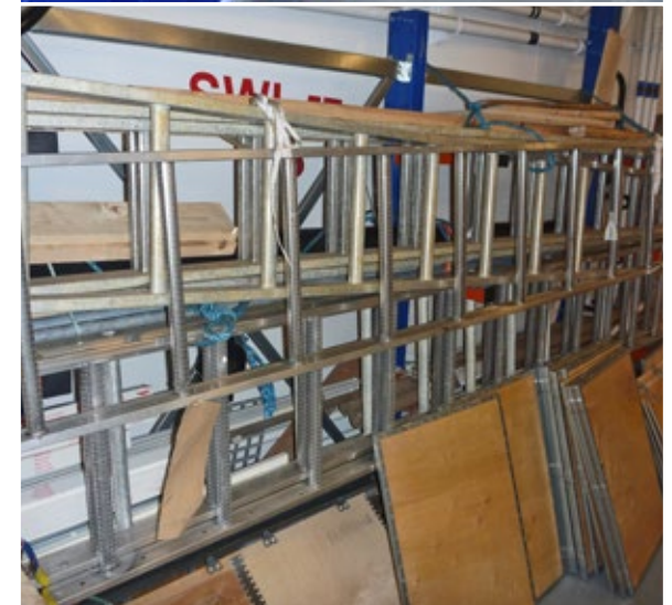
! Portable ladders should be stowed where protected against impact and ideally not exposed to weather.
