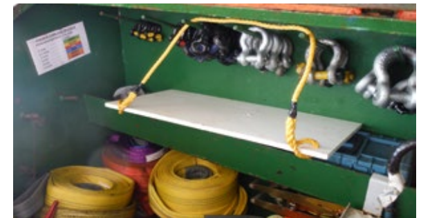
! Shackles marked with colours to indicate SWL/WLL and year of last inspection.
