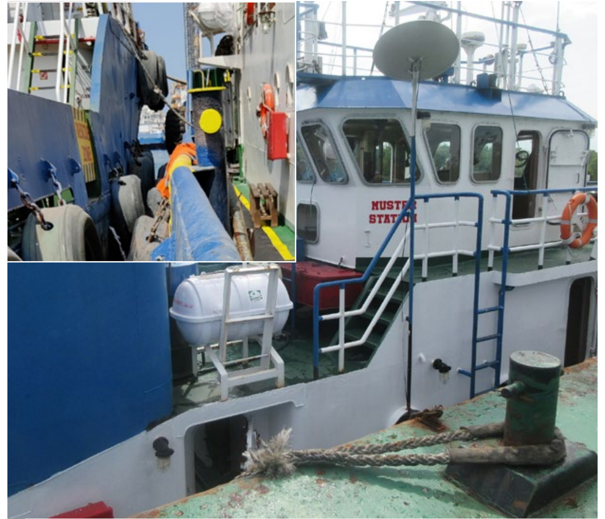
! No means of safe access has been provided.
