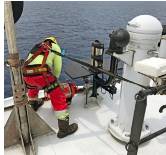
! Examples of a fall restraint system in use. It's not possible for the crewmember to step over the edge.
