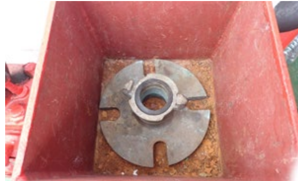
! International shore connection (ISC) connection not kept together with gasket bolts, nuts and washers.
