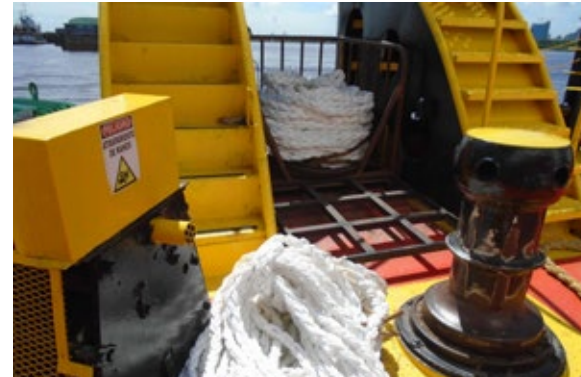
! Ropes stowed off deck but not protected from sun and weather.
