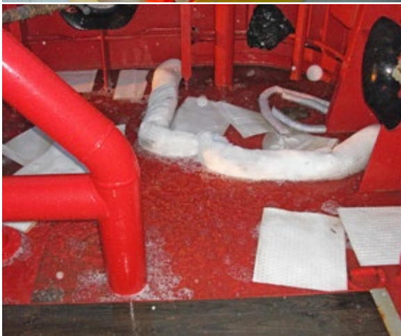
! Adequate SOPEP equipment readily available on deck.
