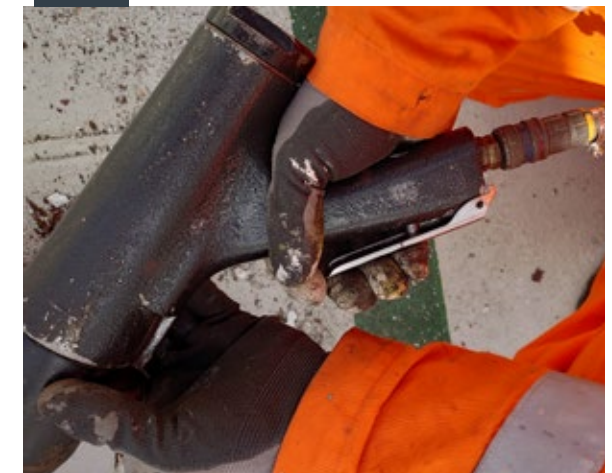
! Spring-loaded switch on the needle scaler is functional (not secured in ON position).
