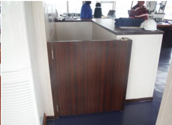
! A crewmember may fall down the bridge staircase during heavy weather or during hours of darkness. A gate at the top of the stairs and/or low lighting on the staircase can help prevent falls
