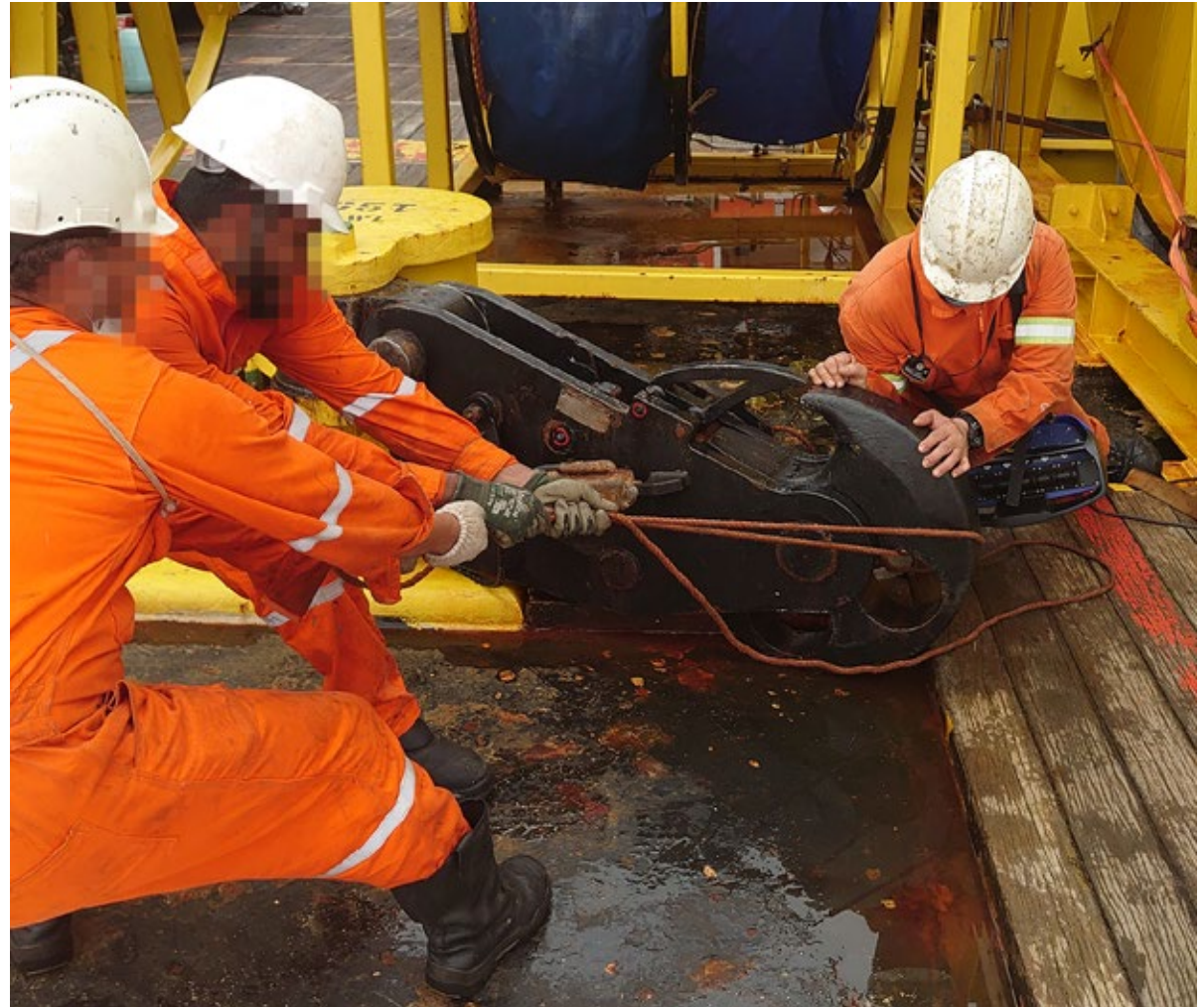
! Crew re-setting the quick release hook on completion of a training session utilising both local and remote (bridge) control.
