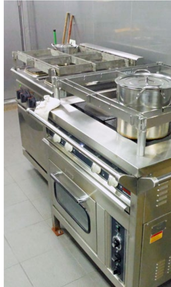
! Galley stove fitted with storm rails and grab bar.
