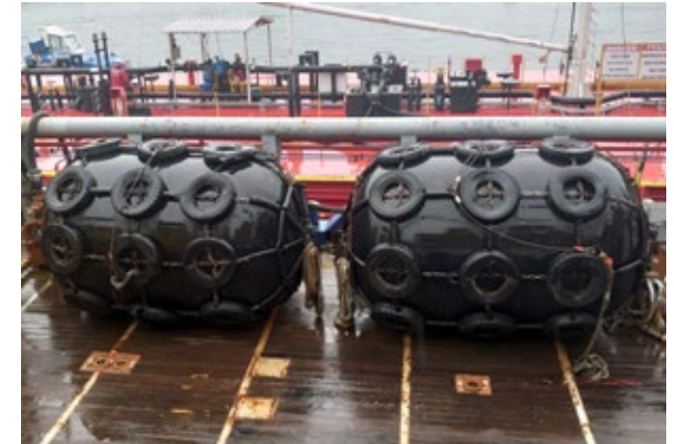
! Pneumatic fenders should be lifted from the lifting points at either end – not from the tyre and chain net. They should be lifted with certified slings or stops.
