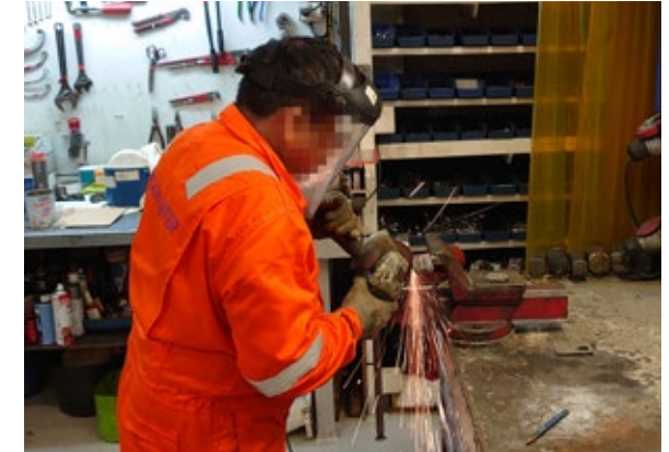
! Safety guard fitted on angle grinder and face shield and gloves in use.
