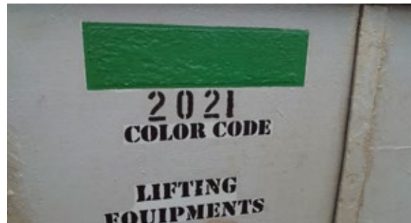
! It is recommended to use a colour-coded system so crew can easily identify the last annual inspection performed on items of loose lifting gear.
