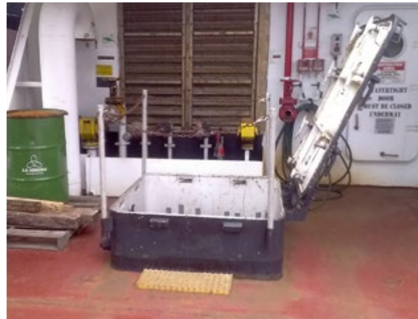
! Stanchions and chains/bars readily available at low level hatches, and tape used in other areas to control access
