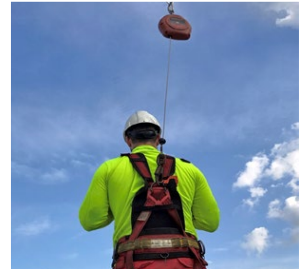
! Use of a fall arrest system, which arrests the user after they fall.
