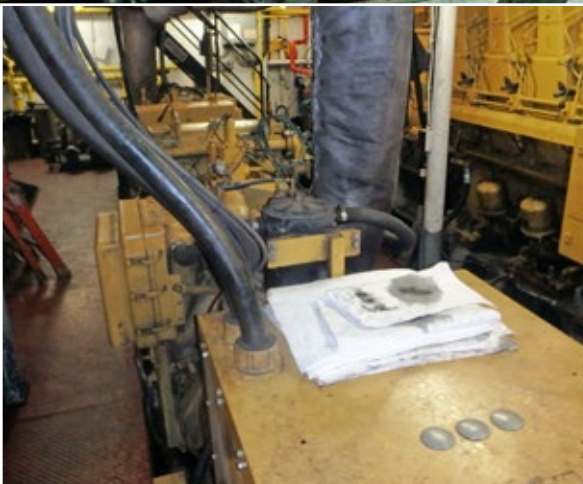
! Oil-soaked insulation should be replaced
