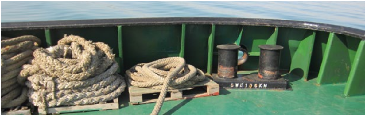
! Ropes stowed off deck but not protected from sun and weather.
