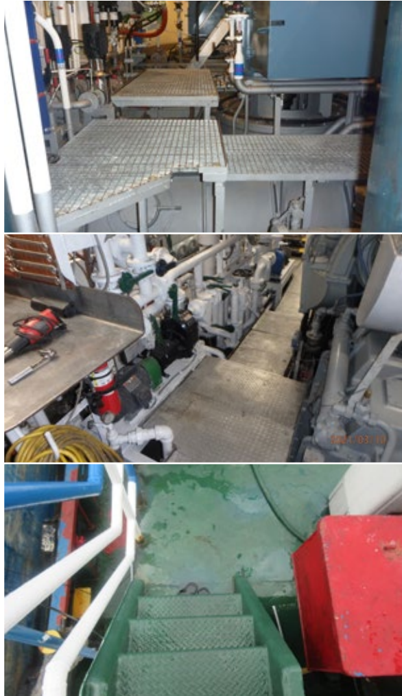
X Inadequate highlighting of changes in deck level
