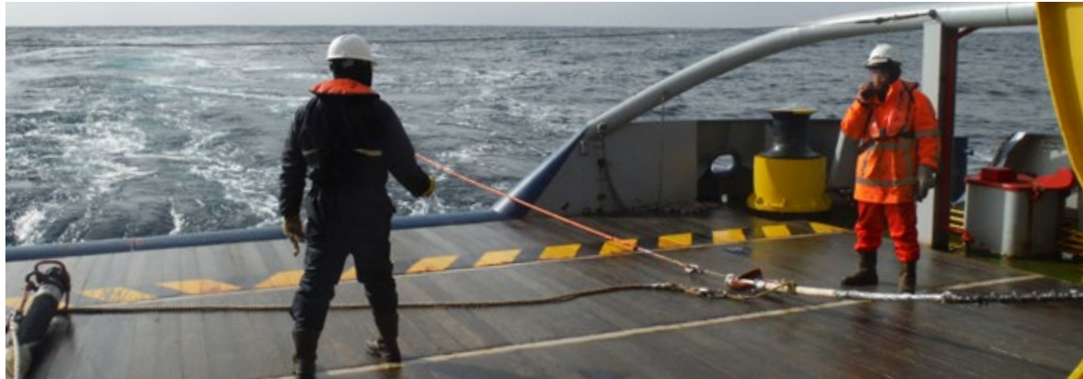
! PPE lines marked on deck. Lifejackets required when working close to the open stern.
