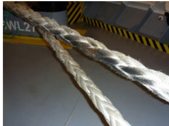
! Ropes allowed to be squeezed between the tug and barge will suffer damage.
