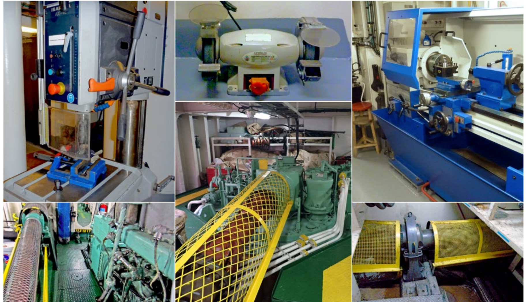
Rotating machinery with guards correctly installed
