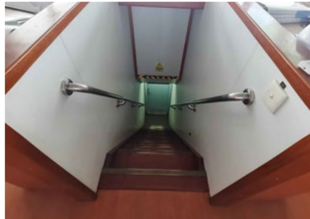
! A crewmember may fall down the bridge staircase during heavy weather or during hours of darkness. A gate at the top of the stairs and/or low lighting on the staircase can help prevent falls
