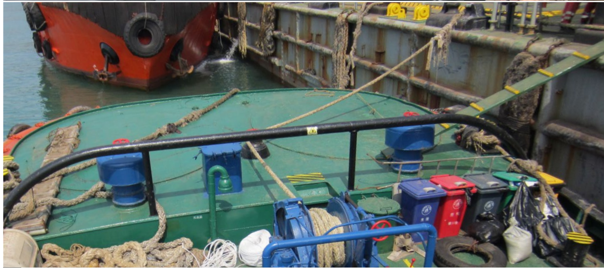
! Gangway brow could be improved by fitting a safety net. The plank with no handholds is unsafe.
