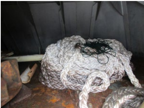
! This rope is soaking up oil from the deck. Oil, paints and other chemical contaminants may degrade the fibre ropes.
