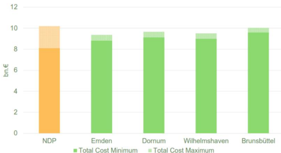
Figure 6-2: Comparison of CAPEX of the German hydrogen network for one pressure scenario with different landing points
