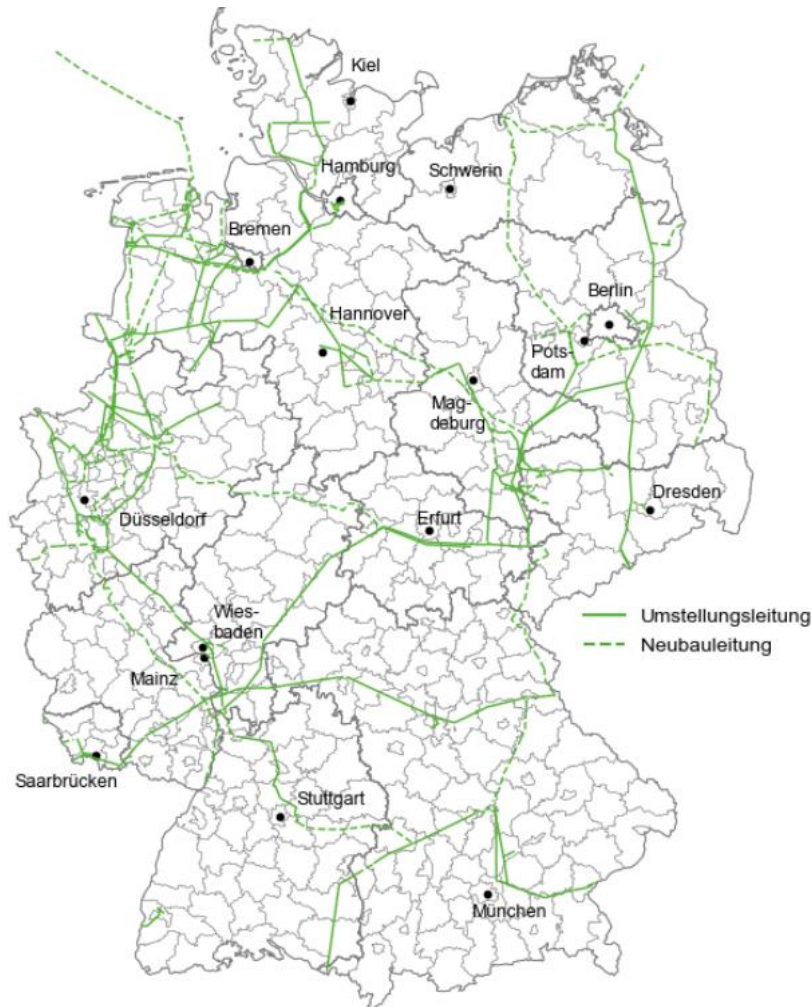
Figure 6-4: Draft map of the Hydrogen Core Network in Germany
