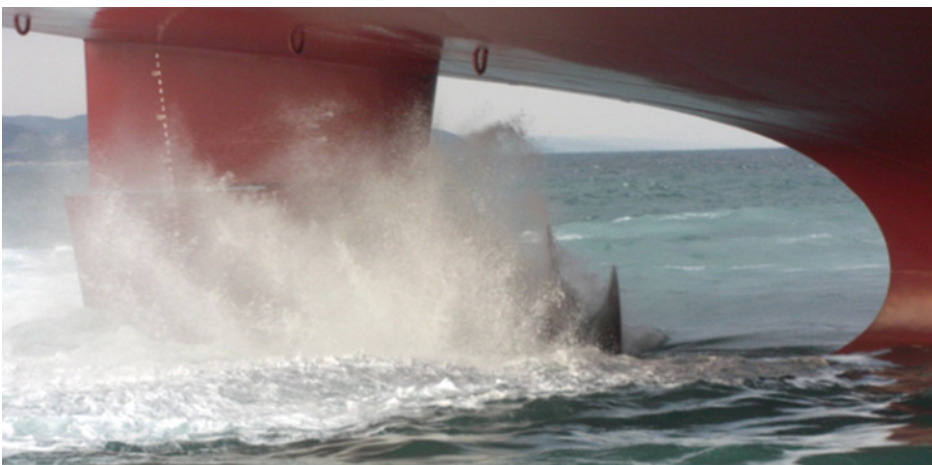
Illustration 2: Incomplete propeller immersion introduces a risk of aft bearing damage
