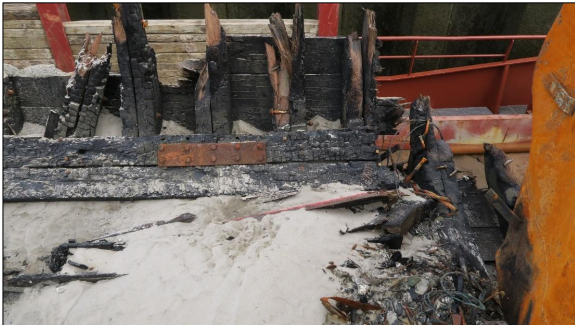
Figure 10: Frames in the area of the fish hold on the starboard side
