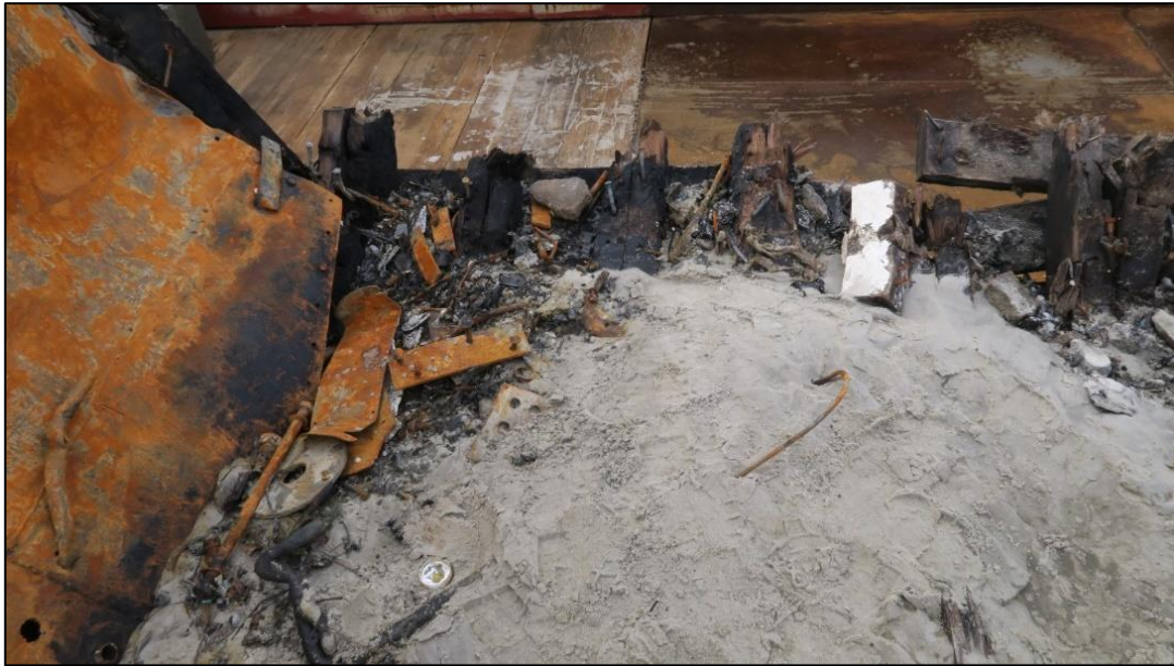
Figure 11: Frames in the area of the fish hold on the port side
