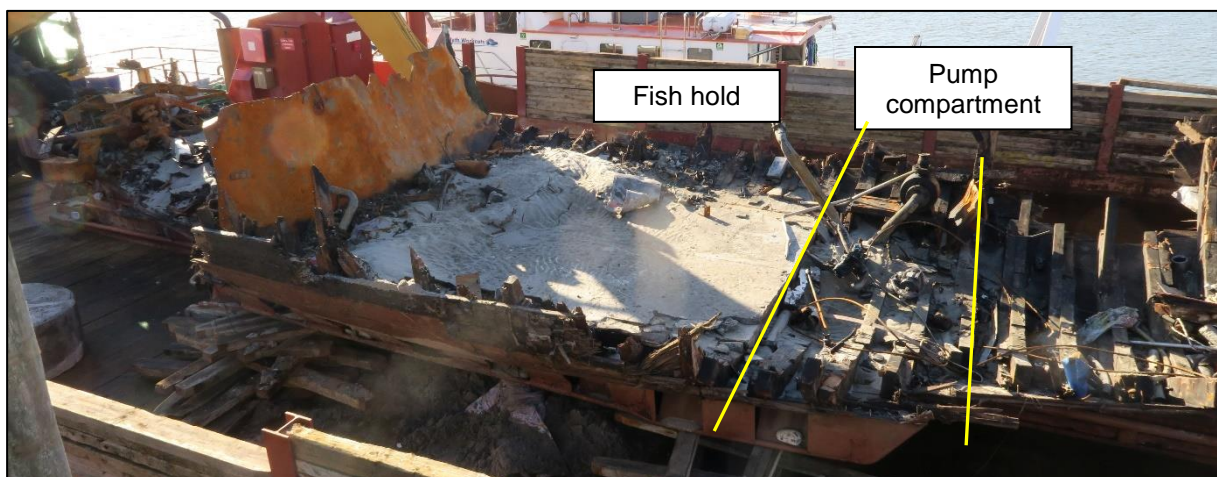
Figure 14: Fish hold and pump compartment
