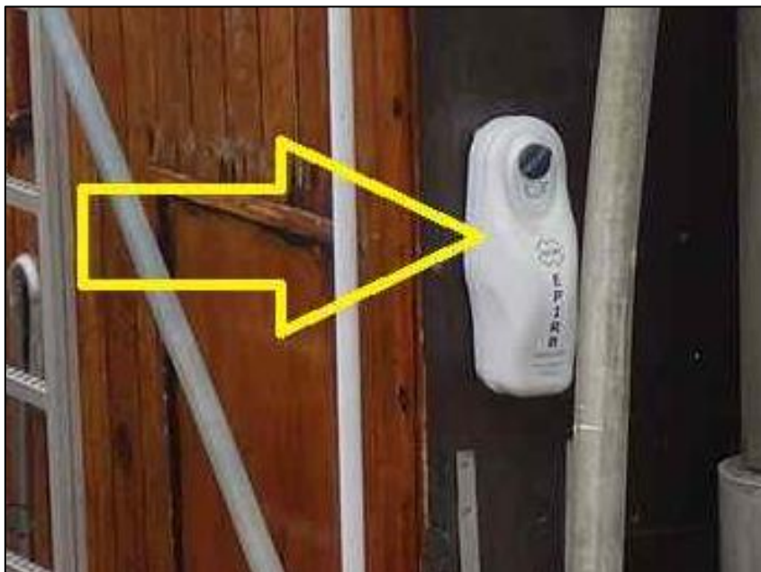
Figure 7: Close-up of the fishing vessel FREYJA's EPIRB
