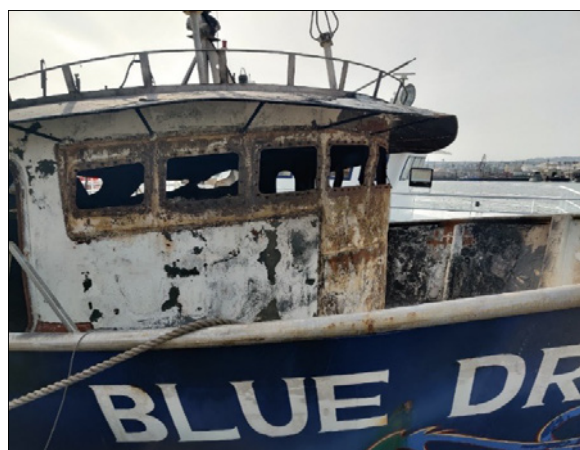
Figure 73. Blue Dragon wheelhouse exterior (top) and interior looking forward (bottom), following the fire. The framing of the false deck below indicates the location of what was the wheelhouse deck. SOURCE: COAST GUARD
