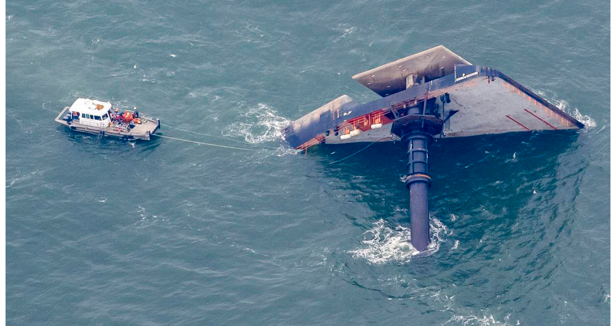
Figure 10. SEACOR Power after capsizing in the Gulf of Mexico when struck by severe thunderstorm winds.
