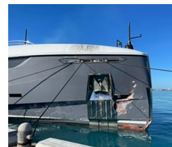
Figure 32. Damage to Utopia IV 's bow. SOURCE: COAST GUARD
