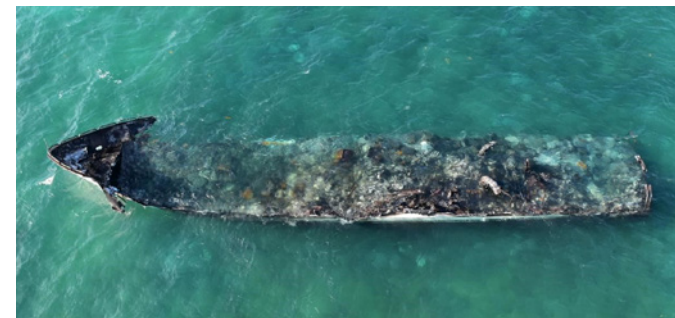
Figure 80. After-fire remains of La Dolce Vita before salvage operations. SOURCE: COAST GUARD
