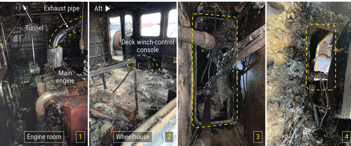
Figure 94. Left to right: Post-fire damage of (1) the engine room, where the crew removed the lagging from the exhaust pipe, as indicated by the dashed line; and (2) the wheelhouse, where the captain observed black smoke emanating from under the deck winch-control console. Damaged pipe/hose tunnel, as identified by dashed rectangles, looking up from the engine room (3), and down onto the deck winch-control console location (4).
