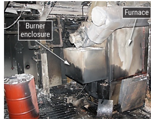
Figure 104. Left to right: Fire-damaged furnace and conveyor belt within the conveyor belt trunk above the furnace. SOURCE: COAST GUARD
