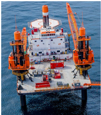
Figure 9. Precasualty photos of the SEACOR Power liftboat lifted, or “jacked up” (left) and under way (below).
