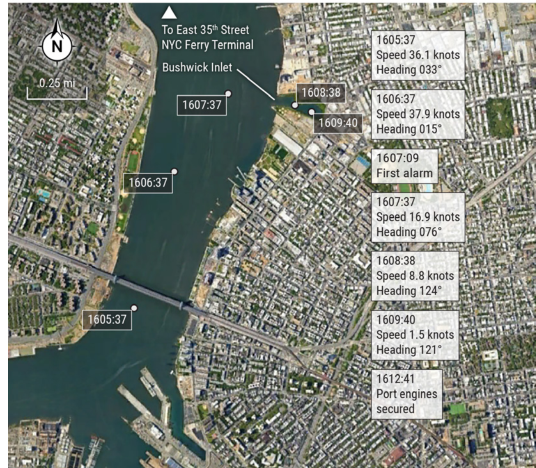
Figure 120. Commodore's position, speed, and heading in the minutes up to the grounding (from AIS). BACKGROUND SOURCE: GOOGLE EARTH
