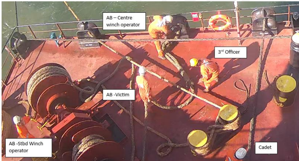
Figure 3. Mooring deck – crew positions during untangling of line
