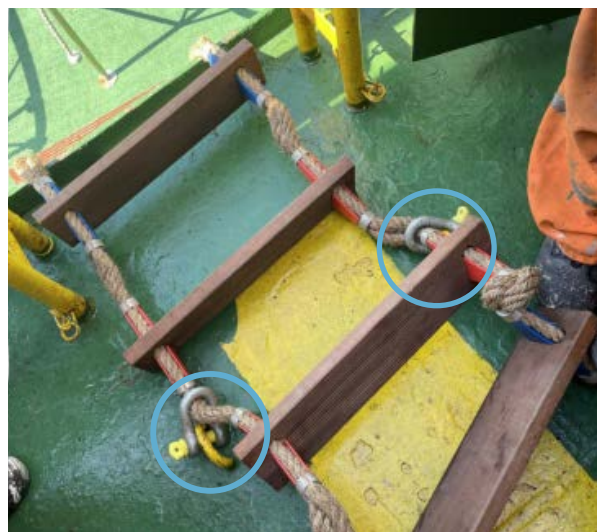
Figure 2: Shackle arrangements (circled) cause the ladder to slip under excessive load when the pilot steps onto it
