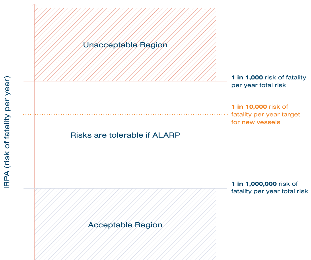
Figure 18: HSE tolerability of risk framework and IMO target value for new ships.
