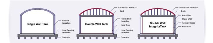
Figure 2.7 Refrigerated ammonia storage tank types
