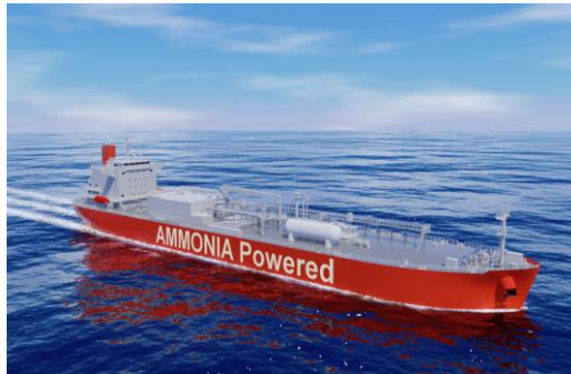
We obtained Approval in Principle (AiP) for an ocean-going liquefied gas carrier fueled by ammonia.
