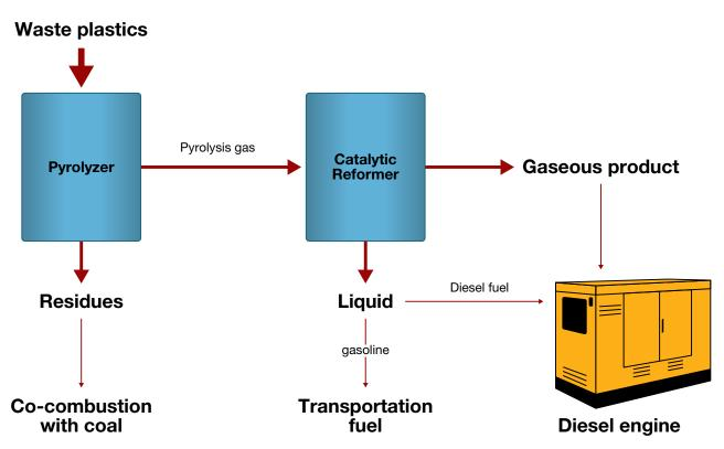
**Figure 15:** Schematic diagram of a system for the conversion of waste plastics into fuels (Source: Syamsiro et al., 2014, 45)
