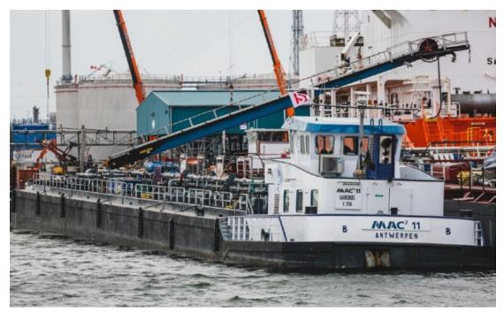
**Figure 9:** Garbage and oily waste collection barge at the port of Antwerp, Belgium (Photo credit: Mac<sup>2</sup>, http://www.mac-2.be)
