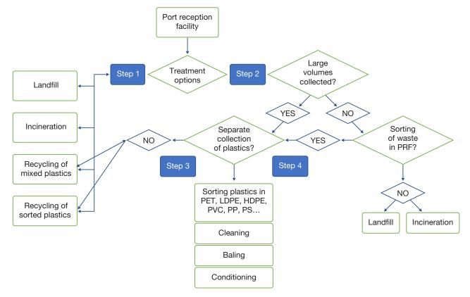
Flow chart 3: Schematic representation of the recycling of plastic into new plastic products
