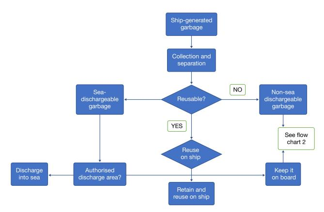
Flow chart 1: Overview of options for onboard handling of ship-generated garbage (Source: Adapted from IMO, 2017, 10)
