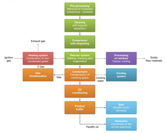
**Figure 11:** Schematic representation of a plastic recycling unit based on pyrolysis technology (Source: Biofabrik, Germany)
