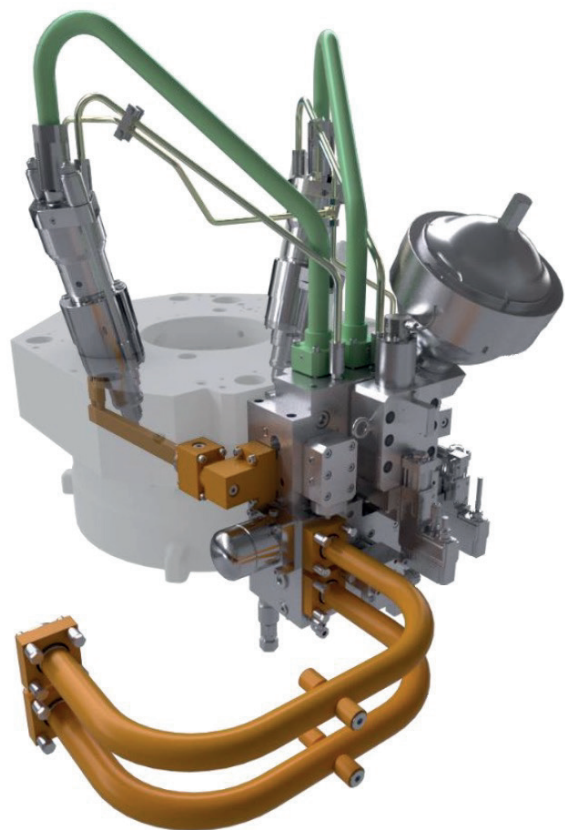
Figure 6.3.3.1: Ammonia cylinder top. Yellow pipes are doubled walled ammonia pipes, green hydraulic pipes for the fuel injectors. Small pipes to fuel injectors are for sealing oil. The big aluminium block is the equivalent to FIVA valves on MAN ME engines (electronically controlled engines)
