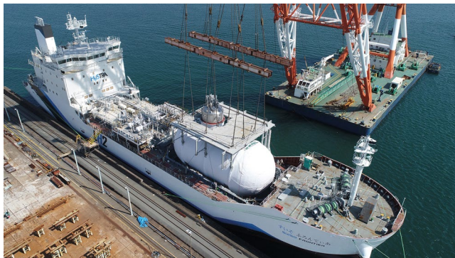
LH 2 storage tank being inserted in the Suiso Frontier (see Bunkering section below) (Source: Hystra)
