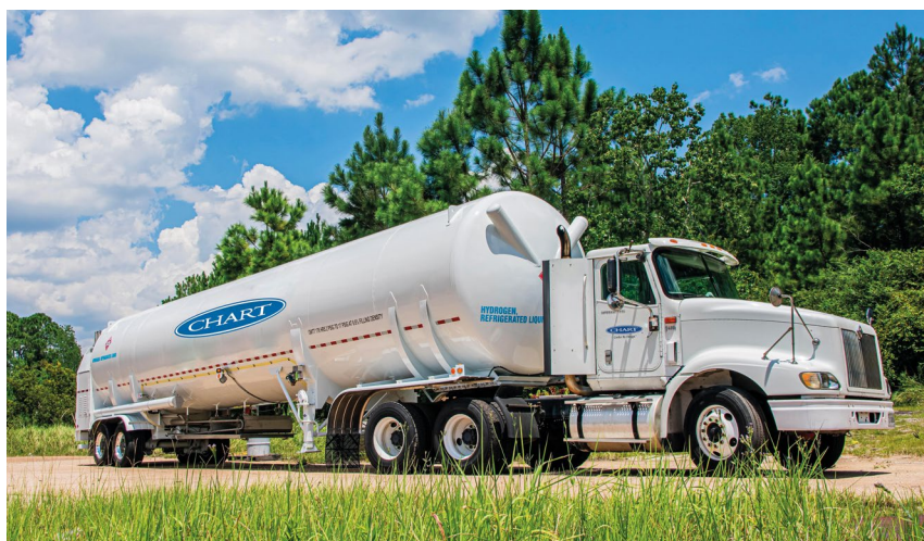
Liquid hydrogen trailer (Source: © Chart Industries, 2022)
