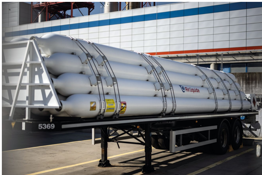
Compressed hydrogen tanks (Source: © Air Liquide)
