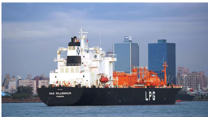
A fully refrigerated LPG / ammonia carrier vessel - The 'Gaz Millennium' (Source: Capt. Jad Ghamraoui, Naftomar)
