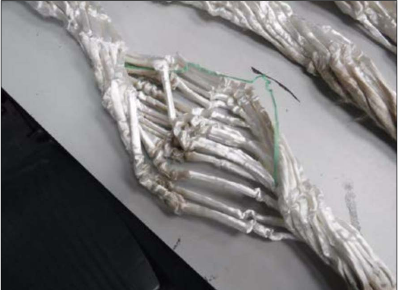
Figure 17: Failed towline pennant yarn kinks
