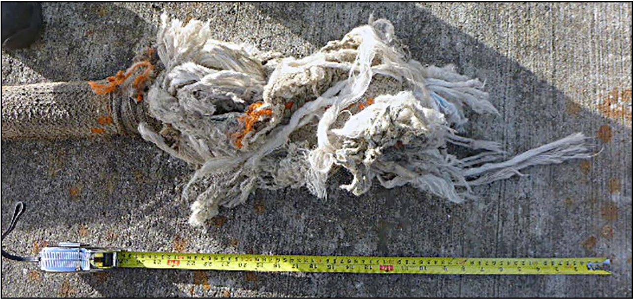
Figure 4: Parted starboard towline pennant
