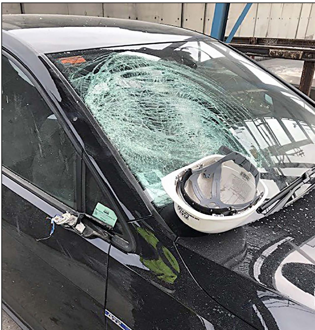
Figure 20: Vehicle laminated windscreen damage
