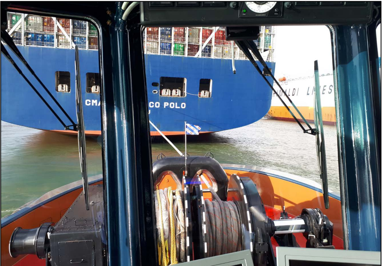
Figure 2: Svitzer Mercurius ' starboard towline connected to CMA CGM Marco Polo prior to failure
