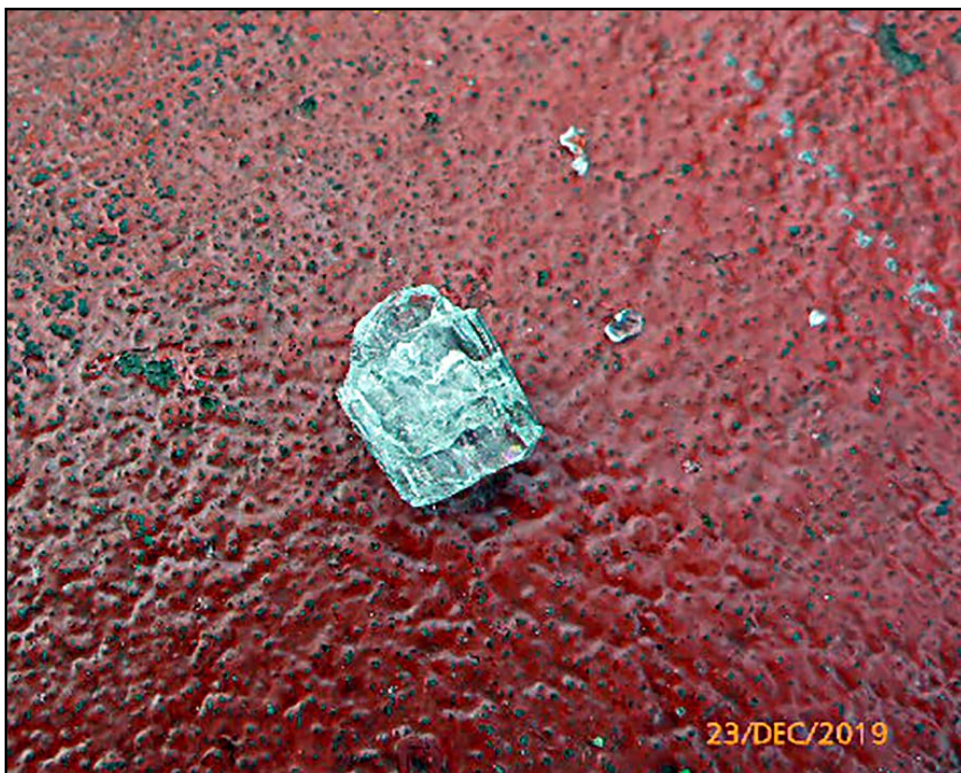
Figure 9: Starboard wheelhouse window glass fragment
