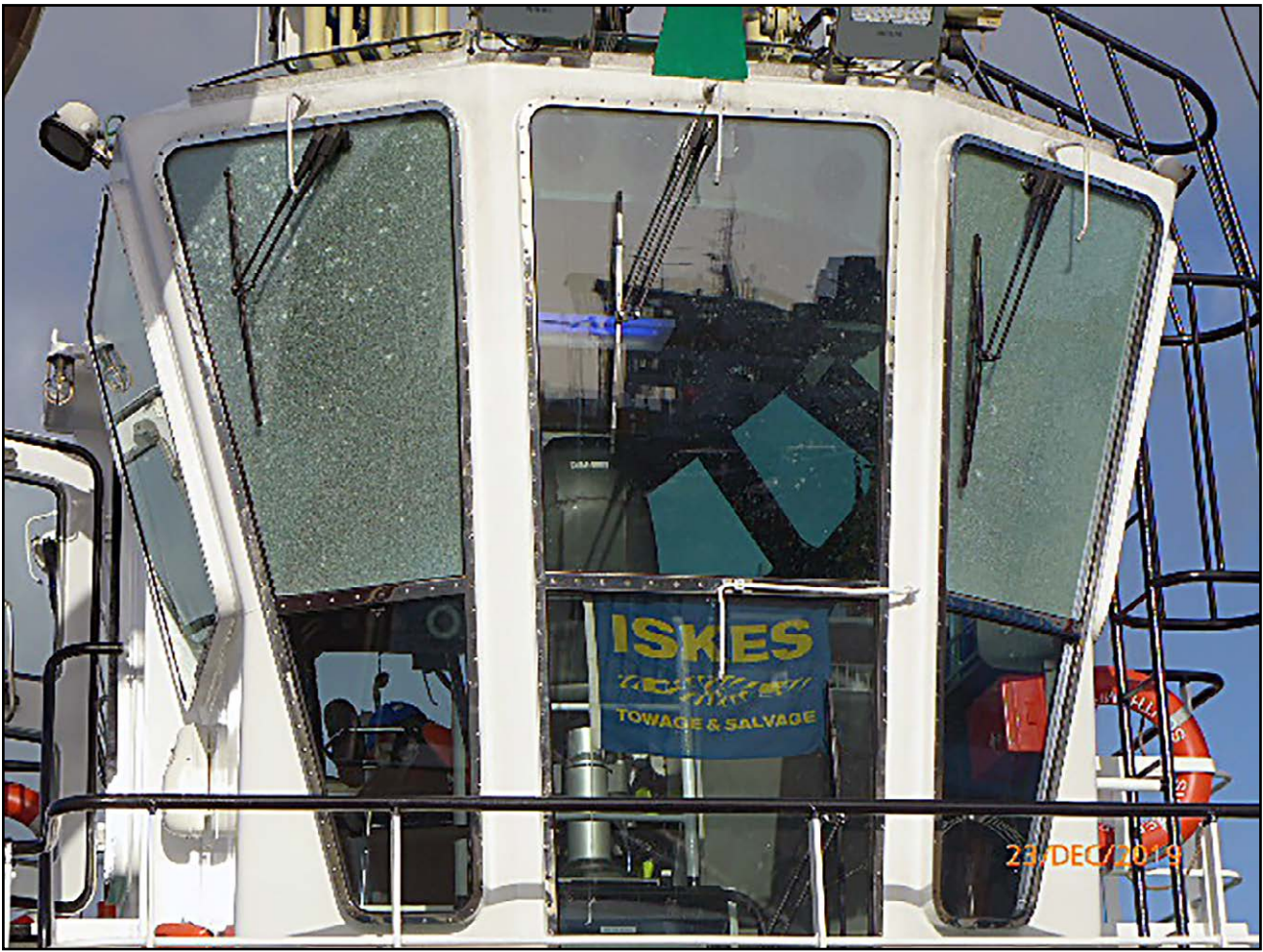
Figure 10: Cracked aft-facing wheelhouse windows
