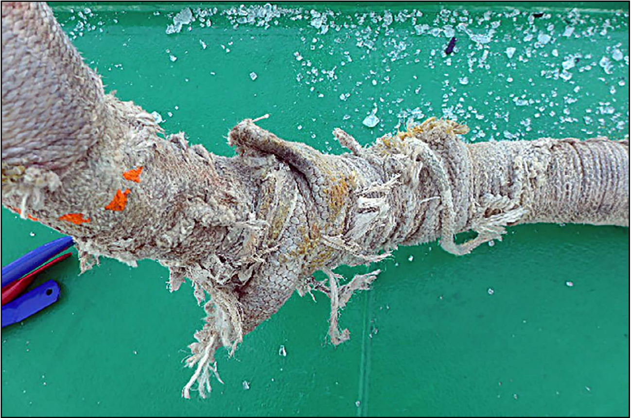
Figure 15: Towline pennant seizing repair
