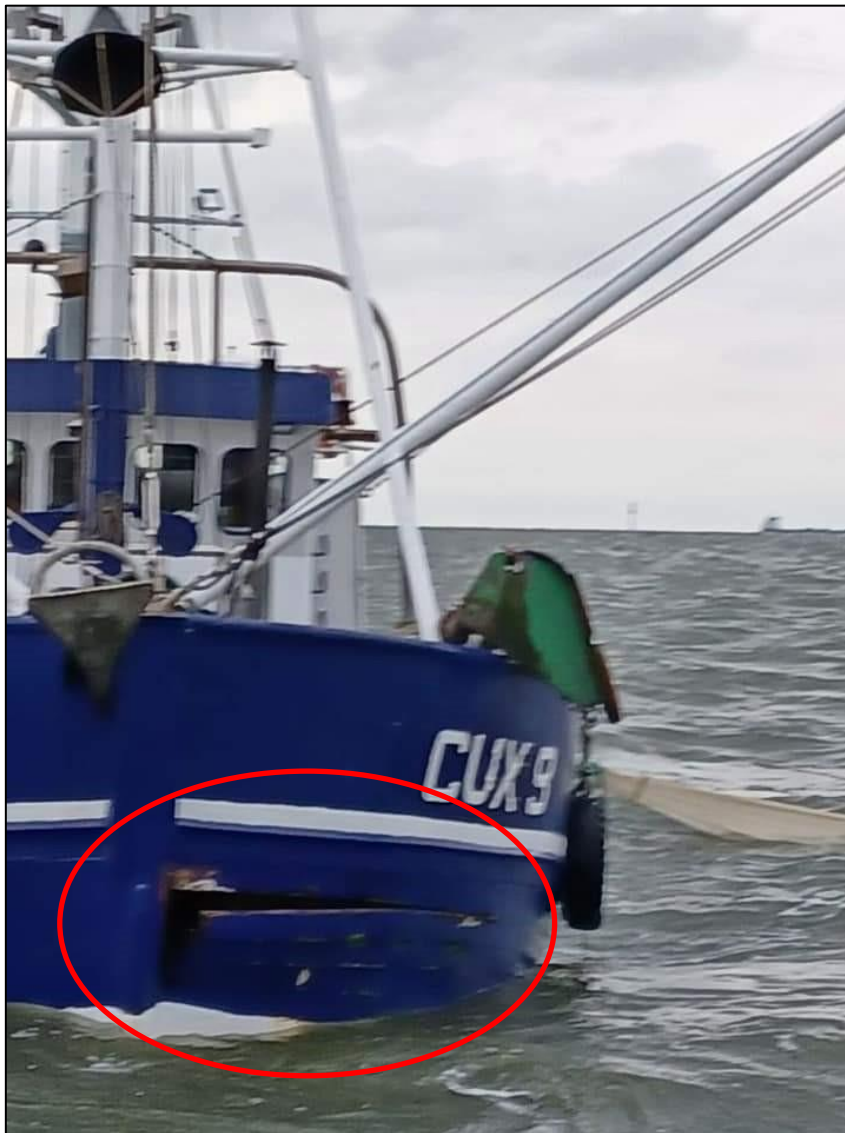
Figure 3: Loose planks at the bow of the RAMONA 4
