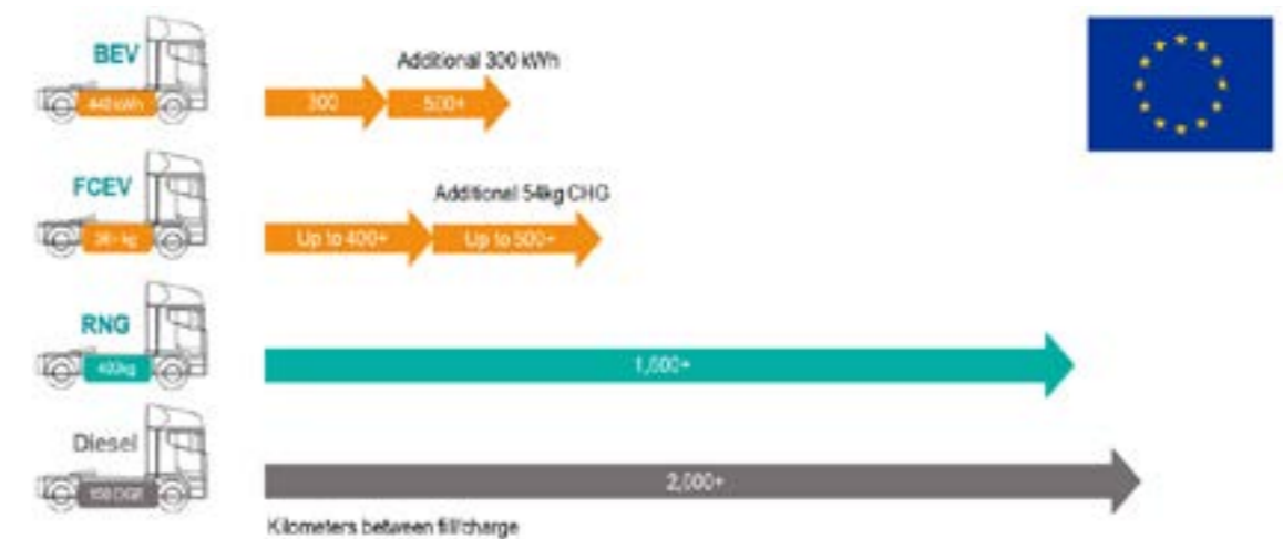
Figure 1: Achievable ranges with different propulsion technologies: BEV (Battery Electric Vehicles), FCEV (Fuel Cell Electric Vehicles), RNG (Renewable Natural Gas) and diesel.
