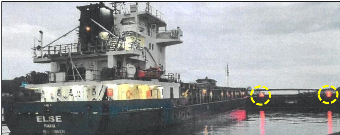
Figure 41: MV ELSE in front of the closed lock gate (red illuminating warning lamps visible) 68
