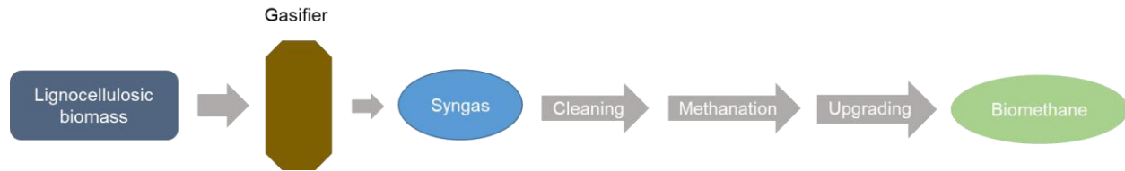
Figure 2.4 - Schematic overview of biomass gasification for biomethane production
