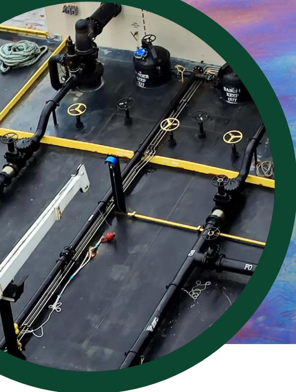
Chief Engineer realised that the oil was escaping from the HFO tank, which was being bunkered and told the duty engineer to transfer all bunker from that tank into another empty HFO tank. When almost the entire bunker had been transferred the trickling ceased.
