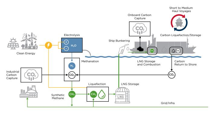
Figure 5: Case Study for CO<sub>2</sub> Carbon Capture on an LNG-fueled RoPax Ferry
